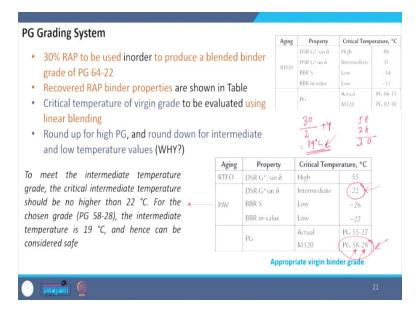
Before we discuss about the second case, there is a note here that to meet the intermediate temperature criteria, or the critical temperature should not be higher than 22 degree Celsius. So, this tells us that though you have got the final grade that is PG 58-28. But this shows only the high temperature and low temperature. It does not tell us about the intermediate temperature.
