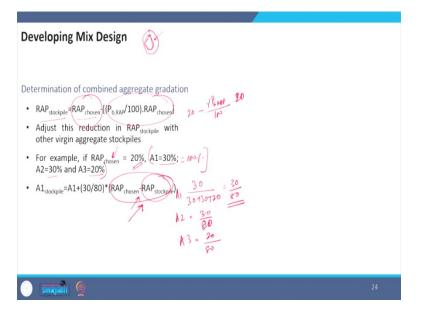
Now, the final steps of mix design that we have to determine the combined aggregate gradation. This is very simple. We have to remember that the RAP stockpile is not equal to the total RAP which is chosen. Because, in the RAP aggregate, we have the binder coated with it. So, we have to remove the binder in order to know the quantity in the stockpile.
