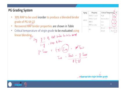
So, let us say that 30 percent RAP has to be used in order to produce a blended binder of grade PG 64-22. So, this is the target grade we are looking at and 30 percent RAP we are utilizing, which means I am trying to find out what should be the appropriate grade of the virgin binder for considering all these three criteria's. Recovered RAP binder properties are shown in this particular table.
