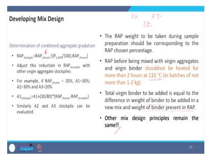
Alternatively, We can do the straightforward calculation, that when we are doing the gradation, we can at the initial stage use the stockpile value and then determine the value of A1 A2 and A3 instead of back calculating and adjusting the gradation.
