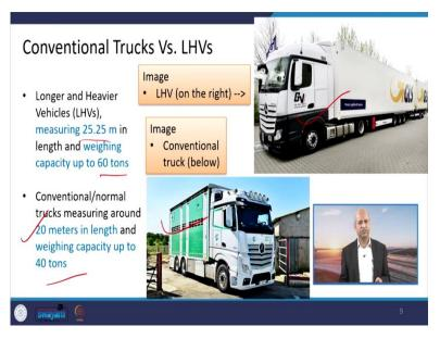
Well, the conventional trucks and these LHVs if you compare then these are the longer and heavier trucks or vehicles and these are the conventional ones. So, you can see the size these are very big as I said around 25 meter and weighing 60 tonnes. Whereas the conventional were 20 meters and weighing around 40 tonnes. So, in weight it is 1.5 times you can say.
