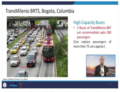
Then these are like one very good example because the two buses they can accommodate around 300 passengers. So, that means, 75 cars, means if we assume that one car is taking around two
