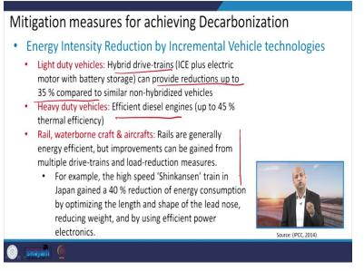
Well, when we talk about mitigation measures for achieving decarbonization, then there are certain ways. Like, we can go for light duty vehicles which are of hybrid nature, IC plus electric motor, battery operated vehicle. We have seen in other presentations also. So, that can really help us to reduce up to 35 % compared to the non-hybridized vehicles. So, that is a good achievement if we go for hybrid vehicles.
