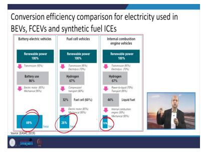
Now, if we compare, like conversion efficiency of electricity used in battery or electric vehicles or these fuel cell vehicles or synthetic fuel ICEs, internal combustion engines, so you can see like overall conversion of the power transmission is 69 %, maximum in battery operated electric vehicles. Whereas in fuel cells it is only 26 % and in internal combustion, IC engines, it is only 13 %.
