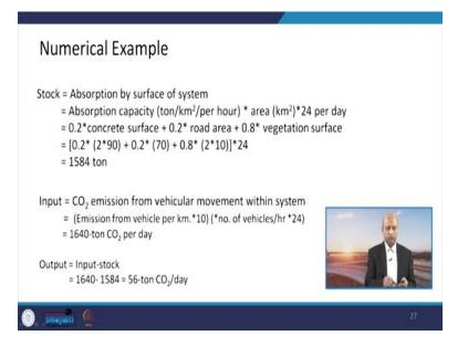
So, simple arithmetic kind of calculations, plus, minus, multiplication, those kind of things are used. You can easily see it. So, those values have been used to calculate how much input is there like 1640 tonne CO2 per day.
