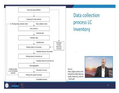
We see the flow diagram of this data collection process for life cycle inventory. So you can see this goal and scope definition we have done, then we do preparation for the data collection, proper preparation is needed, questionnaires are set, then data collection sheet is to be prepared, we do the data collection, then collected data is validated.
