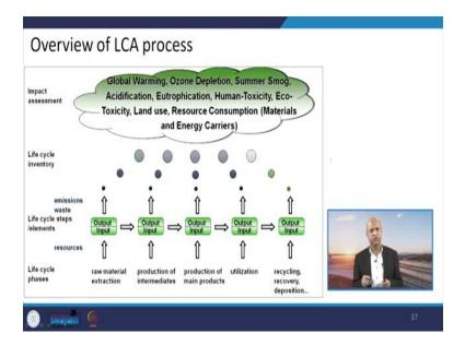
So, in an overview if you want to see the LCA process so you can see like life cycle phases are raw material extraction, production intermediates then main production and then utilization recycling then all these go and they create some sort of input, right?
