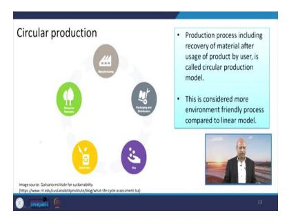
If we see the circular production basically, so this is again the model representation of the LCA, manufacturing, packaging, utilization and end use and again your recovery. So then it is a circular, means just you are discarding something then it is linear, when you are using something, discarded material then it becomes a circular way, because you are using some waste material also as a raw material. So that way the impact will be less, basically.
