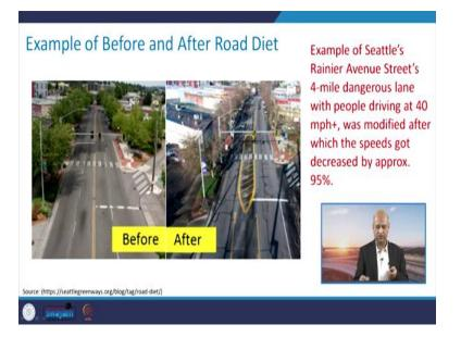
So these kind of road diet structures can be implemented, this was before, this was after. So that can again help in calming down the traffic.
