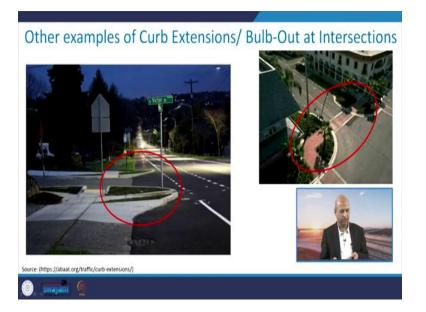
Well these are other examples of curb extensions. So again here very little space is available, so that speed will be not so much and this can be for pedestrians, etc., so that way also these are the spaces which can be used from the main road. So it is narrowing down so here the speed will be automatically reduced and these will be used for other purposes.
