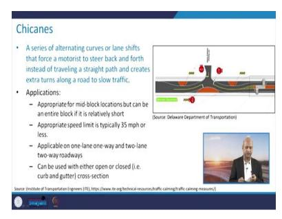
So in that way, then there are structures which are known as chicanes which are nothing but a series or alternating curves or lane shifts, so that when you are going in a zig-zag way then you have to apply the brake, you cannot just go through way. So those kind of structures can be there like this. So that will help again to reduce the traffic speed.
