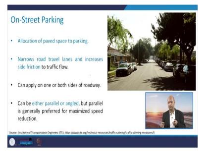
Then on-street parking, also one way to reducing the width of the road and that way the traffic speed will be reduced and this parking can be parallel or diagonal or something like that.
