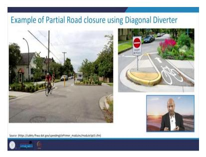
Similarly you can have from the main road you can have this space for this cycle track, et cetera. So the partial road closure using diagonal diverters can be again used for traffic calming, that means reducing the speed of the traffic and encouraging the pedestrians and cyclist movement.
