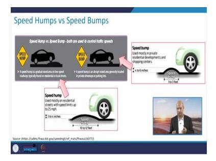
So here it is the difference between speed bump and the speed hump is shown properly, 10 to 12 feet wide and then this height, 3 to 4 inches height. Here it is 4 to 6 inches height, more than the
