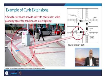
So you can see here, here it can be used for pole also or maybe some benches can be applied if it is needed for old people and so. So a lot of space can be used that way. So these are the ways of the curve extensions, where the narrowing down this street and that way the space can be used more fruitfully. (Refer Slide Time: 28:56)
