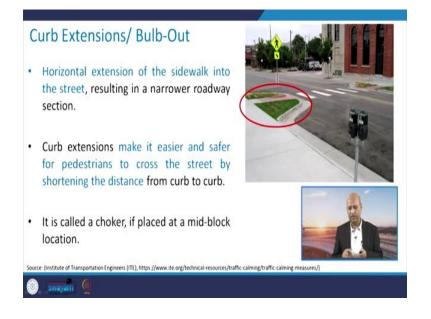
Well there are other ways like curb extensions or bulbing out so that way again for helping the pedestrians, etc., it can be used and that also removes some space from the main road and the speed is reduced by that particular structure.
