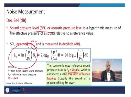
As you know, decibel is the unit and then if you want to convert the sound pressure level, the sound pressure level, so you can this SPL can be measured or denoted by Lp and Lp can be represented by the ratio of the this square sound pressure and reference sound pressure.
