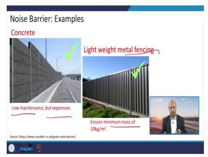
Well concrete structures maybe good in low maintenance kind of but they are expensive when we are constructing and I mean it is difficult to afterwards when if you want to change the location
