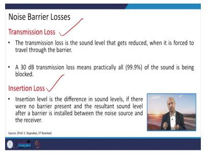
Well, noise barriers losses are there two types like transmission losses because of distance etc., it loses, sound loses the energy and this insertion losses, which are depending upon the initial sound and the sound which is reaching there, so that because of barrier presence that lot of difference is there, which is known as the insertion losses. So, these losses sum up and we get the net result of low sound.
