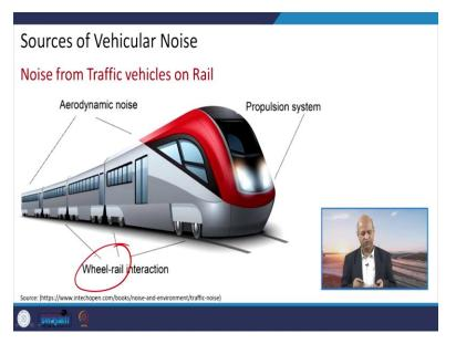
Similarly, like aerodynamics noise because when air is striking or hitting the body and that body also then release some sort of noise, so the propulsion systems and the wheel and road interaction like in case of car or in case of these road vehicles, the interaction of wheel and road is there, so that cause noise, similarly in trains the wheel and rail they also cause, they also produce some sort of noise.
