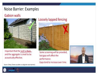
Similarly, again this wall thickness is good and that is a good solid wall with aggregate etc., that will prevent you from the noise, but these kind of screening with gaps will not help as we have seen.
