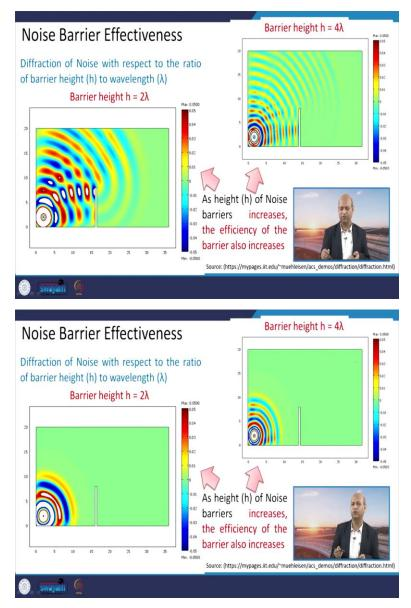
Well, this is like one barrier means barrier how to use the barrier, for example this is the barrier here and as noise is going to this side, so it loses its energy because of barrier height and in next slide you will see that we increase the height of the barrier from this must to four times then how this energy level reduces because of different heights.
