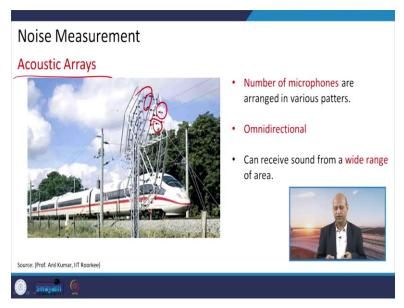
Then these kind of acoustic arrays are used for capturing the noise in and around of a particular site location, so these kind of several sensors can be used for catching the sound, a wide range of a spectrum of the sound.
