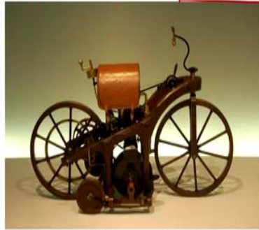
Daimler's and Maybach's first motorcycle. The 'Reitwagen'
