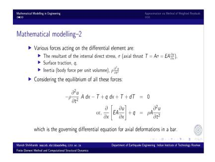
You can see the various forces acting on this differential element. So, the axial thrust is area times the direct stress and that is of course, equal to by making use of Young's modulus and Hooke's law.
