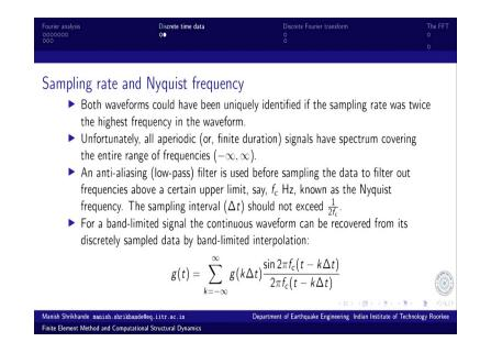
So, both wave forms could have been uniquely identified if the sampling rate was twice the highest frequency in the wave form. So, that is sampling frequency was twice the highest frequency in the wave form. So, that is what we saw. Unfortunately all wave period aperiodic or finite duration signals have spectrum covering the entire range of frequencies that goes from - infinity to + infinity.
