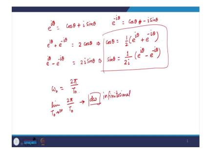
So, I use these two expressions in the Fourier series expansion replacing  $\Theta$  by j  $\omega_0 t$  and I have this complex representation and that I use substitute in the Fourier series and that gives me that brings us to this for particular formulation. So, that will be from j is equal to 1 to infinity, so this is of course the constant term. So, all terms involving cosine and sine they can be represented as positive exponential and negative exponential and terms a and b can be combined.
