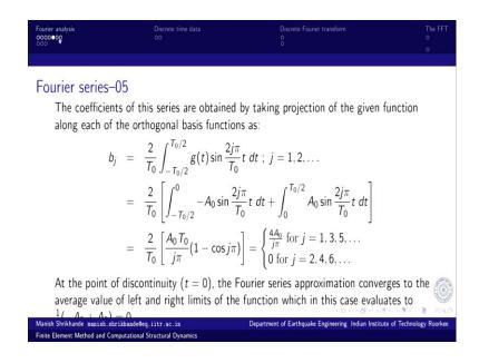
So, in this case we have been looking at this square waveform the Fourier series expansion of square wave form and we found that it is an odd function and it involves only cosine terms and the coefficients of the cosine term b j they can be given as 4 times  $A_0/j$  pi for odd number of harmonics odd or odd harmonics j is equal to 1, 3, 5 and they are 0 for even harmonics j is equal to 2, 4, 6 etcetera. And at the point of discontinuity
