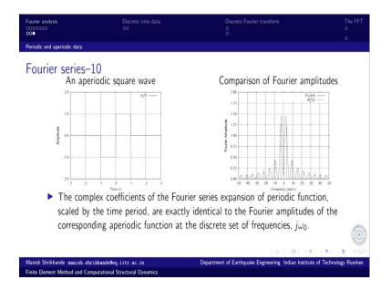
And we can find this these are the Fourier amplitudes that we have. So, we have this we know that this amplitude Fourier transform. So, we are plotting here only the modulus of the Fourier transform complex number with respect to frequencies. Now, as we know from the previous result that for a periodic function it is going to be continuous function and this is what that continuous function is so the Fourier amplitudes.
