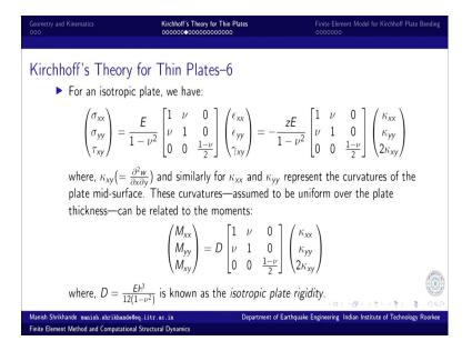
So, for an isotopic plate, isotropic medium we can relate stresses to strain using plane stress I mean so this is where plane stress assumption comes in for plane strain this matrix would be different. So, we as we said plane stress conditions are have a better agreement with what we observe in during experimental studies experimental observation and therefore, we stick to plane stress assumption.
