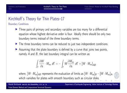
So, this integral can be defined as again integrating this in the boundary integral as assuming A and B are the points. So, if I integrate it along this boundary A to B then this is what it becomes by again using the divergence theorem, and then this is the boundary term and this is the evaluation of these limits.
