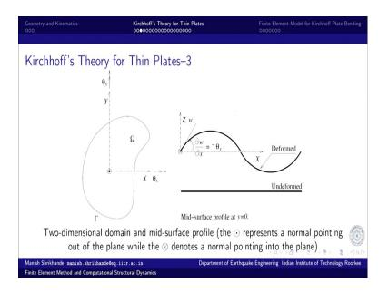
So,  $\frac{\partial w}{\partial x} = -\theta_y$  that is rotation about the y axis and similarly  $\frac{\partial w}{\partial y} = \theta_x$  that is the rotation about X axis. And that imposes I mean this equality imposes the constraint of vanishing shear strain.
