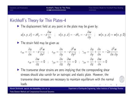
And that is what is given I mean this is similar to what we have in case of Euler Bernoulli beam, this axial strain is proportional to the distance from the neutral axis and we can have compression above neutral axis and tension below neutral axis in case of a sagging moment. And similar kind of geometry is defined for plate accept that it will be now in 2 dimensions.
