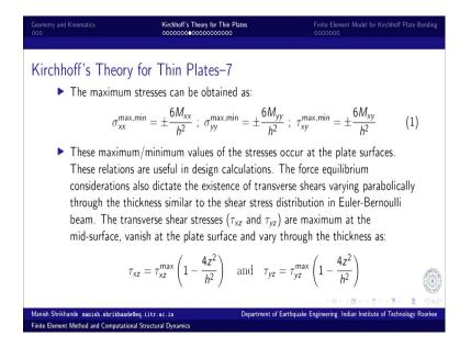
So, maximum stresses can be obtained by evaluating these at values of z = + or - h / 2 and they can be related to the moments. And maximum minimum values of stresses occur at the plate surfaces and these relations are of course, useful for design calculations. Once we have the moment then we can simply find out what is the maximum stress of respective stress I mean direct stresses and shear stresses.
