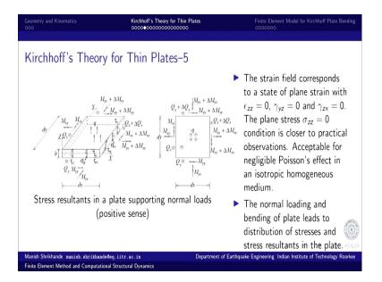
So, these are the stress resultants in a plate, simple I mean these are all the forces that can exist and based on these stress resultants we can impose by considering the equilibrium of forces. I mean force equilibrium and moment equilibrium we can develop the governing equation.
