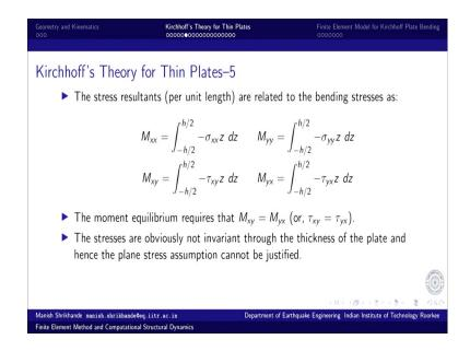
So, these are the stress stresses and these are the stress resultants that we have. So, bending moments stress resultants per unit length are obtained from the integration I mean the of the stress field with lever arm z and integrating over the thickness and we get the M xx and M yy and then twisting M xy and M yx.
