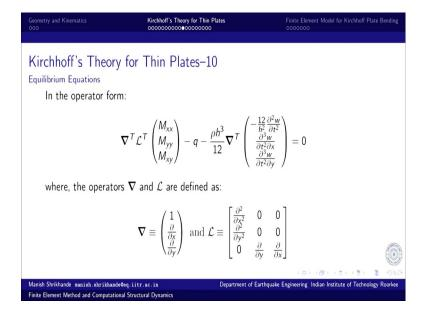
In operator form we can relate these two moment and curvatures moments and the applied forces, and where this nabla is the just the gradient vector and L is the differential operator involving curvatures defining curvatures.
