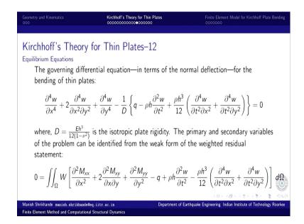
So, eventually we come with the governing differential equation in terms of normal deflection of the plate and that if we substitute for moments in the moment equilibrium equation then moments are proportional to the curvature. So, that is second order derivative of normal displacement or transverse displacement. So, that is so in terms of displacement it becomes a fourth order differential equation.
