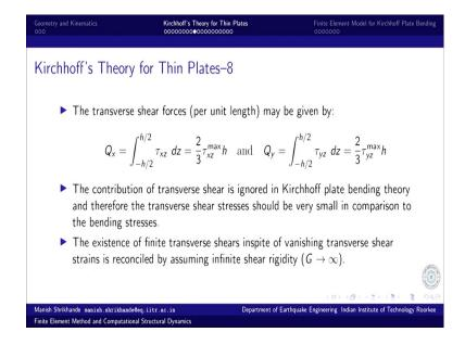
And once we integrate these transverse I mean we can find the resultant transverse shear forces and they can be represented as representative value of a scale down of maximum shear stress and that would be multiplied by thickness and two third of that; that is what it works out. So, these are again transverse shear forces that are going to be used for our equilibrium equations.
