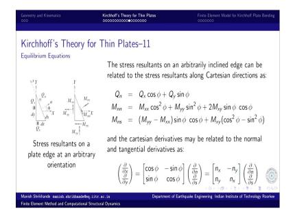
So, far we developed it for edges plate edges oriented along the frame of reference. So, x and y coordinate axis I mean if the plate dimension plate edge is oriented arbitrarily for any arbitrary orientation where the plate edge is defined by normal n and tangential direction s.
