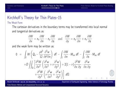
And we can identify we can again transform these into normal and tangential and combine the terms. So, we can have normal derivative and tangential derivative and Qx Qy can be combined to become Qn, Mx Mxy can be combined to become Mnn and similarly Mns. So, torsional and direct rotation.
