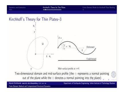
So, this is what the deformation field is. So, theta x that is the rotation. So, this double arrow notation is when the positive sense is when the right-hand thumb points to the direction of arrow, then the direction of curl of fingers is the sense of rotation. So, this is theta x rotation, and this is theta y rotation, rotation about Y axis, if this is X plane X axis and this one is Y axis.
