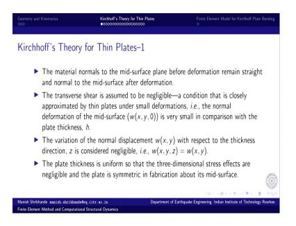
And of course, the variation of normal displacement with respect to thickness is 0. So, there is no variation. So, along the z direction, it the transverse displacement w along z displacement along z axis is invariant with respect to z. So, w as a function of x, y, and z can be represented as just two-dimensional variation w as a function of x and y.
