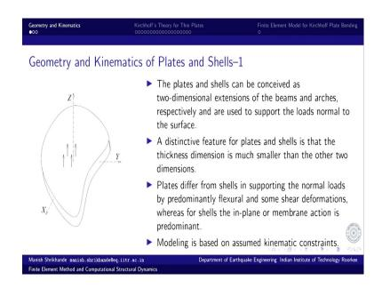
So, what do you see in this is that, it is a two-dimensional extent in X-Y plane, in this case. The dimensions are very large compared to the dimension along the thickness direction, and so, in that respect it seems more close to plane stress kind of situation that we had discussed earlier in continuum mechanics problem. Thickness direction is very small compared to the other in plane dimension in X-Y plane.
