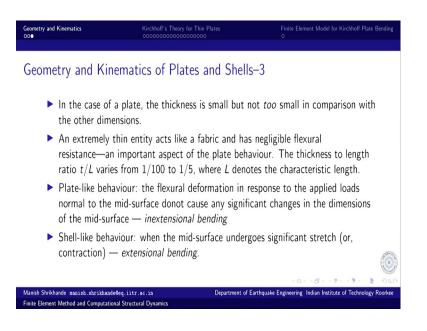
So, an extremely thin entity acts like a fabric, and has negligible flexural resistance which is an important aspect of the plate behaviour. So, as a rough guideline, so thickness to length ratio t by L varies from 1 over 100 to 1 over 5, where L represents the general characteristic length of a plate element.
