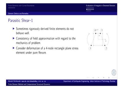
You may look at in this case in this particular case; so, at eta = + or - 1 this has to this has to take the quadratic geometry and at this edge the displacement has to be 0 or on this particular thing the displacements have to be are I mean with respect to x on this edge there is no variation. So, the variation has to vanish in this case on this geometry and similarly for moment applied in this direction it will be the other way round.
