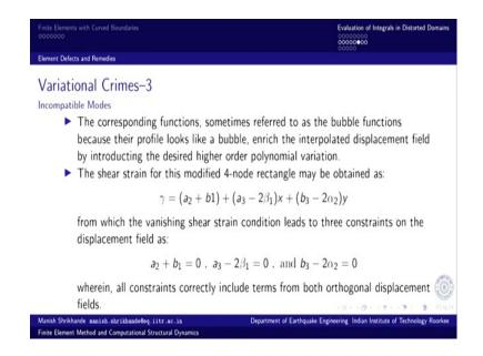
So, these corresponding functions in compatible modes these are sometimes referred to as bubble functions because their profile looks like a bubble  $(1 - x^2)$ , so it is like quadratic and vanishing at x = 1 and x = -1. So, it is looks like a bubble kind of a thing and 1 - y square is bubble like this. So, they enrich the interpolated displacement field by introducing the higher order polynomial variation in the displacement.
