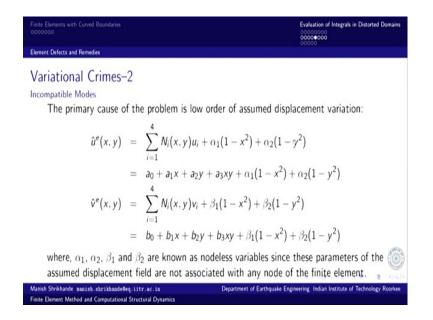
So, the primary cause as we discussed in the modeling of pure flexure by 4 noded rectangle element is the inability to take the curved path and that curvature curved
