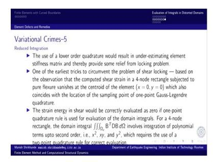
So, at this point centroid of the element the there the shear strain vanishes and the Gauss quadrature one point Gauss quadrature point sampling point coincides with this point centroid. So, if we evaluate the quadrature at this point shear strain would be 0, everywhere else there is distortion shear distortion but at this point this shear strain would be evaluated to be 0.
