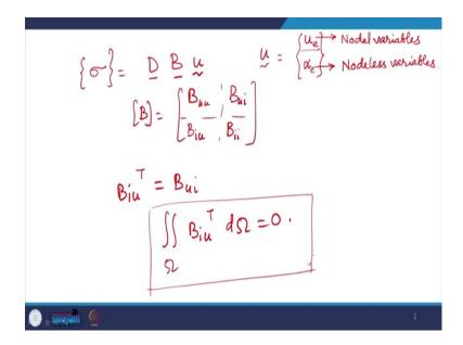
So, stress = D B multiplied by nodal displacement. So, nodal displacement so u in this case = the nodal variables as well as the nodeless variables. So, these are nodal variables and these are nodeless variables and obviously the strain displacement matrix will have some elements which are corresponding to which will operate on these nodal variables and there will be some elements which will operate on which will be contributed by the nodeless variables
