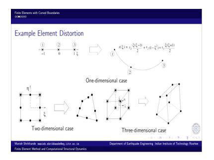
So, this is what we have parent element 3-noded parent element, straight one-dimensional, ranging from I mean this  $x_i$  one-dimension  $x_i$  local coordinate ranging from -1 to + 1. So, node one placed at -1,  $x_i$  is equal to -1 and node 3 placed at  $x_i$  is equal to + 1 and node 2 is the midpoint that is at  $x_i$  is equal to 0.
