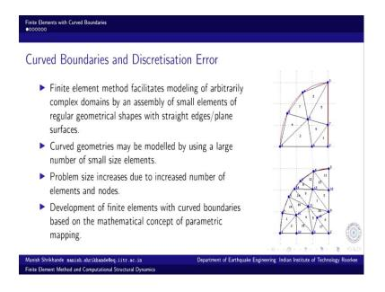
So, just to explain the concept of discretization error and the need for modeling curved boundaries, this one quadrant of a circle; I mean it can be plane stress model or whatever two-dimensional geometry, so one quadrant. And in this case, it is modeled by using 7 finite elements, triangular constant strain triangular constant strain triangle and you can see the discretization error here.
