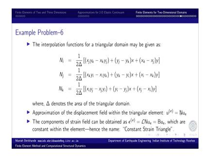
So, for a triangular domain the interpolation functions can again be given in terms of nodal coordinates, as we had seen during this during our discussion of triangular family. So, Ni the interpolation function for ith node that we have, this is the ith node location in the local node numbering for element.
