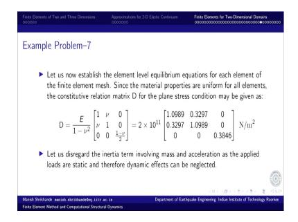
So, in order to establish the element level equilibrium equations, we need the constitutive matrix D for plane stress conditions, what are referred to as coefficients d11, d12, d33, etcetera. So, these are the coefficients of those constitutive matrix.
