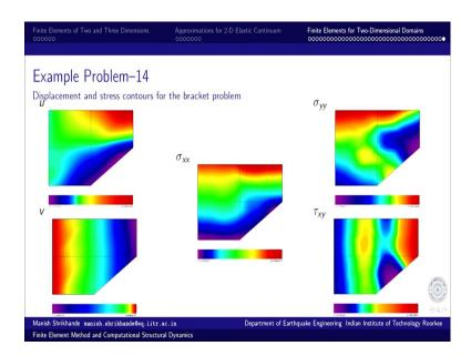
This is the displacement u and v, all through throughout the as a function of x and y. This is  $\sigma_{xx}$ . You can see very beautifully the constant stress, I mean the tension at the top, and compression at the bottom, and very beautifully my color-coded contours can be seen. And this is  $\sigma_{yy}$ , and this is  $\tau_{xy}$  shear stress. And these are just the representative of how the typical results of a finite element stress would look like, a finite element result look like.
