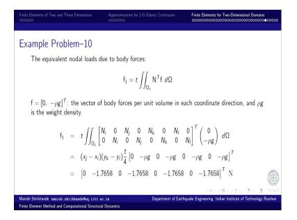
So, this is what the nodal forces will look like, evaluation of nodal forces. So, waiting function multiplication is represented by  $N^T$  f. So, f is the vector of nodal forces. In this case, there is no body force in the along the x direction, but there is a body force component along y direction that is self-weight, and that is referred to here as rho times g per unit volume.
