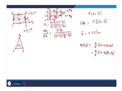
Now, the first derivative is of course, a function of y and the denominator. So, just to tell you, so  $\frac{\partial N_i}{\partial x} = \frac{y - y_k}{(x_i - x_j)(y_i - y_k)}$ . So, it is linear in y and similarly all derivative functions. So, N\_i is essentially (x - xj)(y - yk) divided by numerator normalized at the node (xi - xj), (yi - yk). So, derivative is simply this remaining expression.
