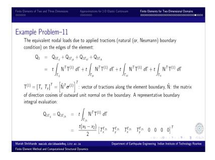
What remains now is this boundaryintegral. How to evaluate these boundaryintegrals? And these boundaryintegrals are again evaluated by segregating the boundaries, looking at each boundary at one time. So, this is gamma ij, the boundaryintegral is evaluated in counter clockwise direction, and in this particular case this boundaryij is common with the boundary for kl for element two. So, the those boundary terms would get cancelled.
