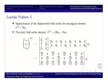
So, the strain field and those derivatives the strain derivatives that these are essentially the derivatives of partial derivatives of interpolation functions. Now, these partial derivatives are completely defined when we specify the coordinates of the nodes. So, for example, Ni is defined by as x - xj multiplied by y - yk divided by xi - xj by yi - yk.
