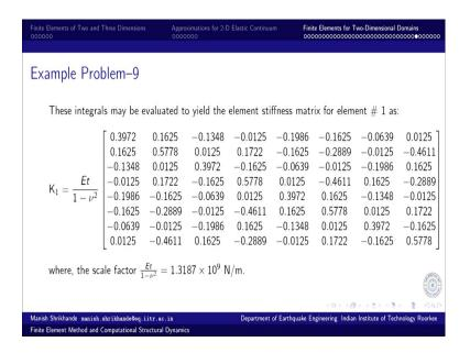
And this is the final integral that stiffness matrix that we have for element number 1. And this scaling factor that we have is based on this Young's modulus and the thickness t of the element and Poisson's ratio nu square. So, this is equal to  $1.31 \times 10^9$  N/m, multiplied by this coefficient matrix 8 by 8 coefficient matrix. So, that defines the stiffness matrix for element 1.
