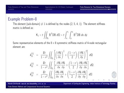
We take element number 1 defined by 2, 5, 4, 1; 2, 5, 4, 1 as the element of our discussion. Process is exactly identical for all the elements. So, we will only refer to this in this discussion. Step by step process for all the elements and in going through the entire every single step, you can see in the solved example in the book that we have my book on finite element and computational structural dynamics.
