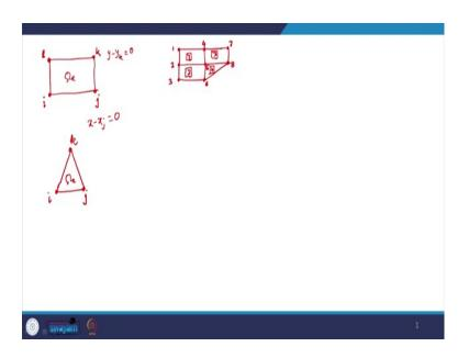
So, what I am referring to here is there are for the rectangle, what we are referring to are these nodes. This node is called i node, this is jth node, this is kth node, and this is lth node, so 4 nodes in all. And as you can see the numbering is always done in counter clockwise direction. And similarly for triangular geometry, this is, so i, j, and k right. So, this is for element one particular element. So, triangular element, rectangular element.
