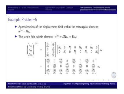
So, using these interpolation functions, we can approximate construct the approximation of primary variable displacement field within the element domain. So, u within the element as a function of x and y is given by interpolation matrix, matrix of interpolation function, nodal variables multiplied by the variable nodal values of the primary variable. And this strain field is of course given by the derivative differential operator on this displacement field.
