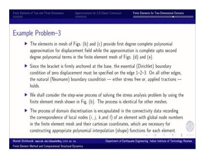
So, elements 4 noded rectangle and 3 noded triangle they divide they provide the first degree complete polynomial approximation for displacement field. And for these 8 node
