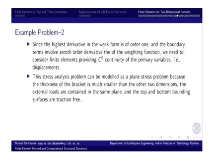
So, C 0 continuity elements are required, primary variables. And primary variables or of course, the displacements along x and y direction, and x direction we consider it to be in this direction and this is of course y. So, x and y; x is along the length span of the cantilever, and y is transverse direction.
