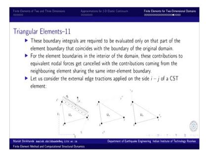
And only the boundary term has to be evaluated when it is coinciding with the domain boundary. So, the boundary integrals are required to be evaluated only and on that part of the element boundary that coincides with the boundary of the original domain. So, element boundary is the same as the part of the original domain boundary. Of course, one element cannot cover the entire domain boundary.
