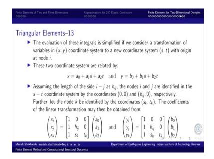
And that we will do by defining the linear mapping. So, evaluation of these integrals is simplified if we consider a transformation of variables in x, y coordinate system to a new coordinate system s, t with the origin at node i. So, for each edge we take it one at a time.
