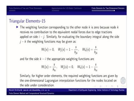
So, the weighting function corresponding to other node k is 0 because node k receives no contribution from the equivalent nodal forces due to edge traction because edge tractions are only coming on the node i, j. So, the other node does not really matter.
