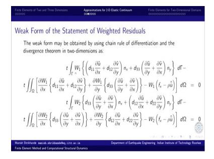
This is the boundary integral. So,  $\Gamma$  is the integral of the element that we have. So, how do we evaluate these boundary integrals?
