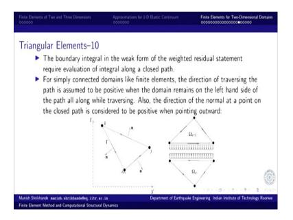
And it is to be evaluated along the closed path. So, this is the boundary integral that is to be evaluated in the closed path. So, I go from i and j. So, that is and from j to k and from k to i and that is the normal outward normal positive direction and the outward flux is of course, going positive outward normal.
