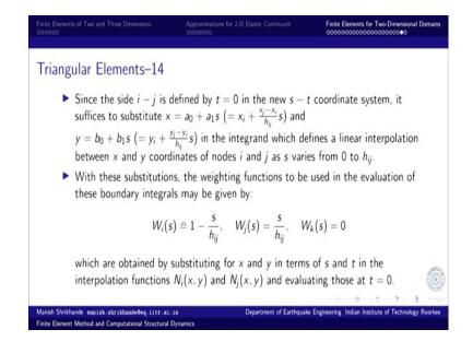
And since side i-j is defined by t is equal to 0 in the s-t coordinate system it is sufficient to substitute x is equal to linear function of s and y as a linear function of s; and t is obviously 0. So, no point in adding that term no additional benefit. So, it is a linear interpolation as you can see it is a linear interpolation between x y coordinates of i and j
