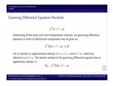
And that governing differential equation in terms of deformation can be given in terms of a differential operator that relates strains to displacement L. So,  $L^TDLu$  is the vector of deformations plus f is the vector of distributed body forces along each component oriented along respective coordinate directions, and this is equal to the rate of change of
