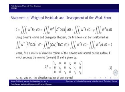
And then we develop the statement of weighted residuals and develop the weak form of the statement of weighted residuals. So, this is the weighted residual statement. W is a weighting function. Please note that  $R_{\Omega}$  here that we are looking at is a vector with three elements; there are three relations in each coordinate direction. So, this is in a sense a set of simultaneous differential equations.
