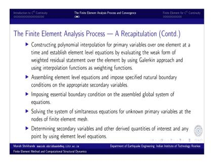
Then we construct polynomial interpolation for primary variables over one element at a time. Establishe the element level equations by evaluating the weak form of weighted residual statement over the element by using Galerkin approach and using interpolation functions or the shape functions as the weighting functions. Once we have these element
