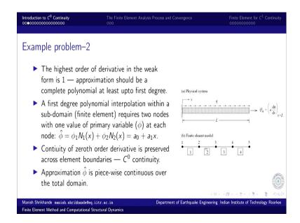
Now, for these simple problems that we have seen here we only referred to the finite element mesh, which was only straight line. The entire problem entire domain was a straight line. All the elements that we used (four elements) were in the same line. So, the same frame of reference could be used for defining the element level equations for all the elements, but that is not true in general.
