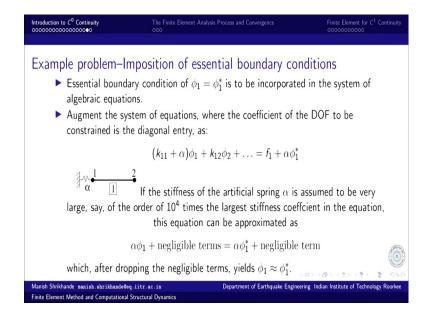
And once the element level equilibrium equations are established those are assembled into a global system of equations. After the global assembly the specified essential boundary conditions are imposed using this very simple penalty function approach or the stiff spring approach.
