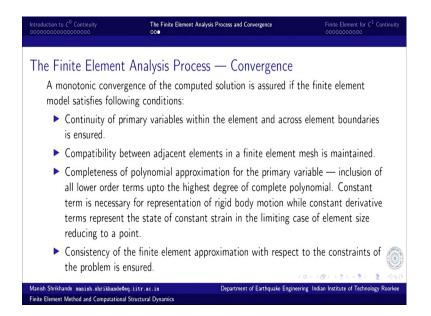
The first requirement is of course, continuity of primary variables within the element. Within the element the variable that we are approximating has to be continuous. This is automatically achieved by using interpolation model. And because we are using interpolation model and different elements connect with each other through shared nodes and the primary variables at those nodes are also shared. So, the continuity of the primary variable is also ensured across element boundaries.
