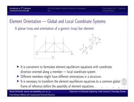
And we may have elements with arbitrary orientation. For example, a simple truss bridge as shown in figure above. This planer truss comprises of several bar elements which are interconnected through hinged connections and they together support the transverse load. These kind of structures are very common in the truss bridges. These different elements have different orientation and obviously, it is easier to define the element level equations when the axis is oriented along the member length.
