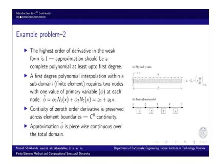
And we are discretized this domain 0 to L into a set of 4 finite elements, 2 noded element. Each element comprising of 2 nodes and equi spaced. We considered to keep simple matter simple because the geometry is uniform distribution is uniform. So, there is no such need for any different discretization. So, we divided the whole domain into equal parts, 4 equal sub domains of L/4 lengths each were quarter of length.
