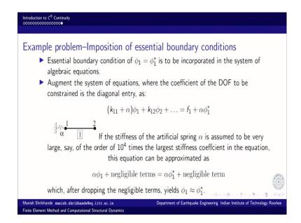
And, we can then proceed with the imposition of boundary condition. Now, natural boundary condition we already applied. The essential boundary condition is that is we need to apply phi at x is equal to 0, it has to take some prescribed value. So that value has to be specified. So, let us say that value is phi 1 star. That has to be incorporated in the system of algebraic equations.
