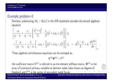
And this is by substituting second equation for second equation substituting weighting function as N j and again evaluating the same weighted residual statement integrals, we end up with this algebraic equation in terms of unknowns  $\phi_i$  and  $\phi_j$ , and again one
