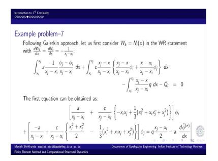
So, this is what by following Galerkin approach using weighting function as the interpolation functions. So, first using  $N_i$  we obtain the first equation after evaluating the integral. We obtain algebraic equation in terms of  $\phi_i$  and  $\phi_j$  and this is the boundary term corresponding to  $N_i$ , W is equal to  $N_i$  weighting function is equal to  $N_i$ .
