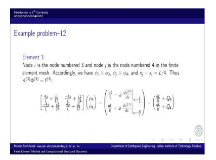
Then we again move the increment the element counter move to element number 3. Now for element number 3 the node i, the left hand side node is node 3 and node j the right hand side node is node number 4 and so on. So, the primary variables are also  $\phi_3$  and  $\phi_4$ , length of the element is L/4, again we end up with similar set of equilibrium equations.
