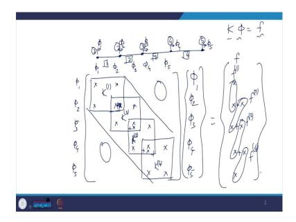
And similarly, for the element number 4 which is defined by nodes 4 and 5 I would have let me just complete the mesh. So, this is element number 3 this is element number 4 and this is node 5; this is node 4  $\phi$  4 $\phi$  5 so node 5 element number 4 defined by these 4 terms.
