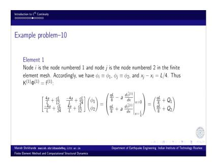
And this is what the equations  $K \phi$  is equal to f for the element number 1. So, K for element 1,  $\phi$  for element 1 is equal to f for element 1. So, these are element level equilibrium equations that have been derived from the evaluation of weighted residual statement weak form.
