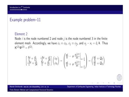
Now, all that has changed is the interpretation of node i. So node i for element number 2, the left hand side node in element number element number 2 is node 2 in the mesh node 2 in the mesh. So, this is what. So node 2 in the mesh is this. So, this is the finite element mesh. So, for element number 1 node i is node number 1, node j is node number 2, for element number 2 node i is node number 2 and node j is node number 3 so on.
