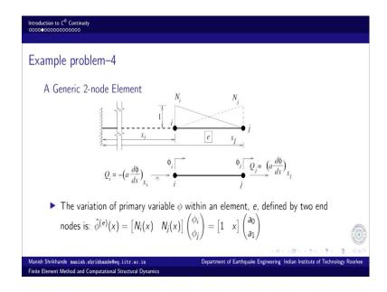
And we saw that after we develop the weak form of the domain residual. We found that it was the first order the highest order term was only the first degree and therefore, only  $C^0$  continuity only the I mean the primary variable is the basic unknown of the problem the unknown function of the problem itself and the continuity of primary variable only is desired and therefore, the zeroth order derivative is required to be continuous, so this is called  $C^0$  continuity.
