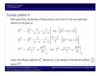
So, generally if I look at the terms. So,  $k_{ii}$  diagonal terms, they are identical if I look at it. If we check these equations off diagonal terms are also identical. So, it is a symmetric matrix and the loading term corresponding to  $i^{th}$  node. We have this simple equivalent, the total intensity q multiplied by length of the element and then equally distributed at
