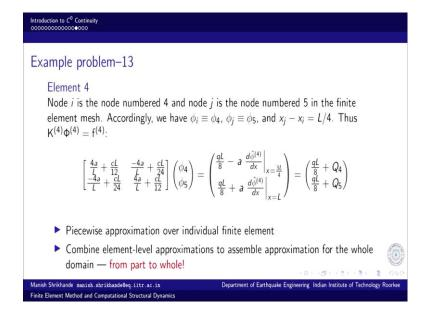
And then finally, element number 4 similarly, defined by nodes 4 and 5 and the primary variables are defined by correspond to the variable at node 4 and at node 5. So,  $\phi$  4 and  $\phi$ 5 and that is what the element level equations are.
