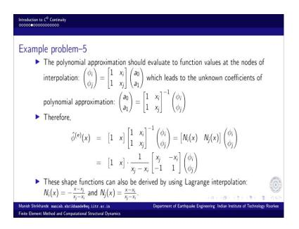
And, this is how by imposing the interpolation condition we can determine  $a_0$   $a_1$  coefficients and the interpolation functions can be derived and they are can be derived by
