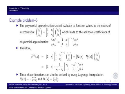
So, the polynomial approximation should evaluate to function values at the nodes of interpolations. We can invert this coefficient matrix of coordinates and a 0 a 1 can be evaluated as simply inverse of this coordinate matrix and the nodal values of primary variables.
