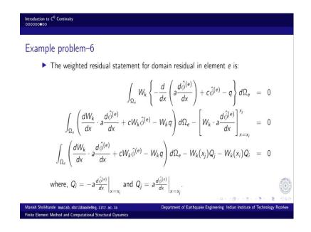
And we go back to the weighted residual statement only the domain residual. We will come to the boundary conditions when we assemble the contribution from the all elements when we look at the complete assembly. So, at the element level we only look at the domain residual in the weighted residual statement. So, when we say domain residual weighted residual statement for the domain residual.
