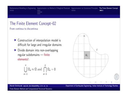
So, what to do? So, the solution is very simple, we divide the domain. So, divide and conquer that always works, this strategy never fails. So, since the construction of interpolation model is very difficult or may well naively impossible for large and irregular domains; we look at the possibility of approximating the total domain by superposition of smaller sub domains and these sub domains are of regular geometry.
