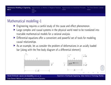
For example, in this case. So, axial rigidity A E is uniform and that is what allows us to construct the same approximation over the whole domain. If some of these things are not uniform; let us say cross section is not uniform or different materials appear in different parts of the domain, so Young's modulus might change. So, in that case it becomes difficult to construct an approximation, which will hold over the entire domain.
