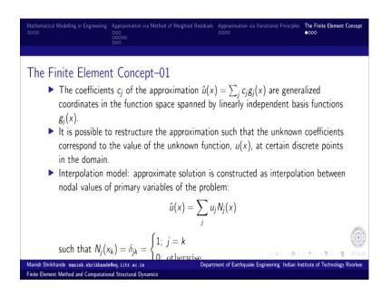
So, we look at another issue that the approximation that is of the form  $c_j g_j$ . The coefficient  $c_j$  they are generalized coordinates of the function space spanned by the basis functions  $g_j$ . So,  $g_j$  they are scaled by these coefficient  $c_j$ . So, individual importance or contribution of individual basis function is scaled by this coordinate  $c_j$ .
