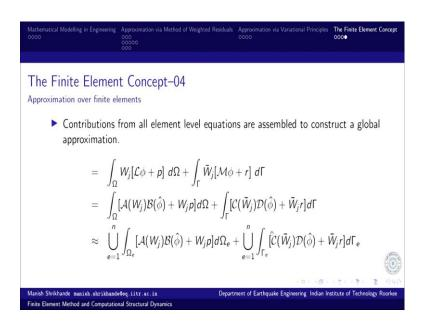
And once we have these element level equations, those element level equations are assembled to construct a global approximation. So, in operator form. So, the total domain represents this domain residual term, weighted residual of domain residual term and the weighted residual of the boundary residual term.
