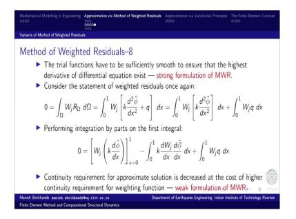
So, now although in the strong form the unknown had to have continuity of at least twice differentiation. In the weak form, the continuity requirement is reduced by one order by at the cost of increasing the continuity requirement on the weighting function. So, this derivative here on the approximation is transferred to the derivative on the weighting function.
