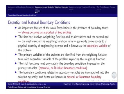
So, the presence of boundary terms that always occurs as a product of two entities and the first one involves weighting function and its derivatives and the second one, the coefficient of weighting function term it generally corresponds to a physical quantity of engineering interest and it is referred to as the secondary variable of the problem.
