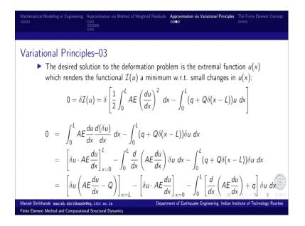
So, now the stable equilibrium configuration would correspond to the variation first variation being 0. So, we consider the variation of this problem. So, desired solution to the deformation problem is an extremal function  $u_x$ . So,  $u_x$  should render the functional I(u) to a minimum. I mean minimum because we know it has to be a minimum potential energy, but first variation only it talks about the stationarity and that is the prerequisite of minima.
