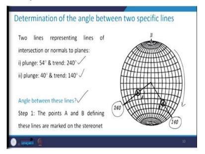
So, here we are taking the two lines with plunge of  $54^{\circ}$  and trend of  $240^{\circ}$ , that is line number 1. Then the second one is the plunge of  $40^{\circ}$  and trend of  $140^{\circ}$  that is line number 2. So, these two lines they may represent the axis of tunnel or anything or they can be the normal to any planes. Now the question is how to determine the angle between these lines? That questions answer that we are going to find out in subsequent slides.
