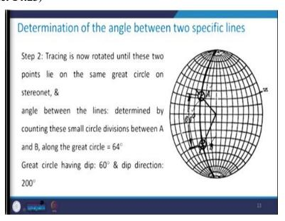
So, what is done in this case is, we need to rotate the tracing sheet in such a manner that these two points which we have marked A and B, they lie on the same great circle. And then what we do is we measure that how many points or how many intervals are there in between these two points along that great circle, not along horizontal direction, not along vertical direction, but along that great circle. That angular distance is going to give us the angle. Let us see how we do that?
