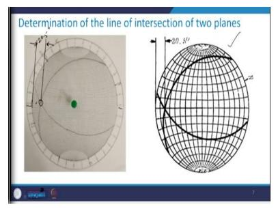
So, this is how we need to do? So, the point of the intersection was this point and we have rotated in such a manner that it is lying along you see this  $270^{\circ}$  and  $90^{\circ}$  point here. Now how to determine it is dip and the dip direction? So, you see from the extreme circle, you just measure of this distance radial distance, this is 10, 20 and little bit more than 20, so that is going to be  $20.5^{\circ}$ .
