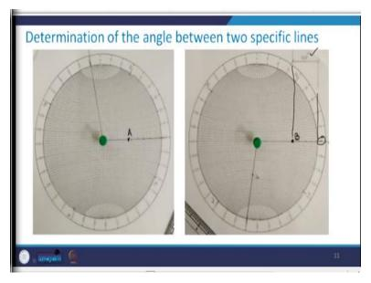
So, what is done here is we have this line  $240^{\circ}$  mark which was there, I rotate the circle, so that that  $240^{\circ}$  is matching here. And then I count from here, like  $54^{\circ}$  was the angle, so 10, 20, 30, 40, 50 and then 2 marks, so I will mark here this as A. Similarly, for this point B again, so I have that two lines, one was for  $140^{\circ}$  and another one was  $240^{\circ}$ , so this is what that we did with  $240^{\circ}$ .
