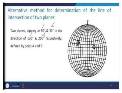
Now there is an alternative method of determination of the line of intersection of two planes. This we have already discussed using one particular method. But using the poles also, we can find out the line of intersection of the two planes. Because I mentioned to you that the planes can either be represented by a great circle or they can be represented by their poles, when we represented it by great circle, then how to determine the line of intersection of two planes that we have already seen.
