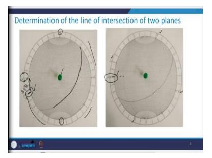
So, this is the one plane which we already have seen in the previous class how to draw. This is the one plane. Now see north is coinciding with 0 here and it is in the original position which is pinned at the centre. So, from here in the clockwise direction I come and then I mark a point as 250° having the dip direction of the other plane. Now the next task is going to be this 250° mark which is there I need to rotate it in such a manner that it coincides with this west direction or 270°.
