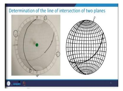
See, this is what that we have done. So, corresponding to this  $30^{\circ}$ , I draw another great circle which will be representing the plane having dip as  $30^{\circ}$  and dip direction as  $250^{\circ}$ . And obviously, this plane is having  $130^{\circ}$  dip direction and  $50^{\circ}$  dip as we have seen in the previous class. So, we have these two planes, so this is how it will look like, this is here your north is there south east and west.
