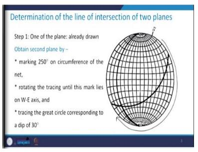
What we need to do is, we need to measure  $250^{\circ}$  along the circumference, then we need to rotate it in such a manner that it coincides with west east axis and then we will trace the great circle corresponding to a dip of  $30^{\circ}$ , let us see how we do this.
