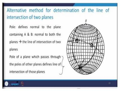
Then because this pole defines normal to the plane which is containing these two planes, that is A and B. So, which is normal to both the planes, so that will give us the line of intersection of these two planes. So, the pole of a plane which passes through the pole of the other planes define the line of intersection of those planes. So, please remember this, this is a very, very important statement.
