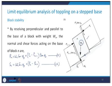
Now, by resolving the perpendicular and parallel to the base of a block with weight  $W_n$ , the normal and the shear force which will be acting at the base of the block, they can be obtained as
