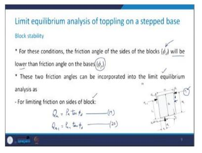
So far such type of conditions, the friction angle of the sides of the blocks is being represented by  $\phi_d$ . This will be lower than the friction angle on the base which is  $\phi_f$ . Now, these 2 friction angles can be incorporated into the limit equilibrium analysis as we are going to discuss. So, for the limiting friction on the sides of the block, we can write that  $Q_n = P_n \tan \phi_d$
