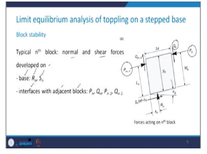
Now, let us consider a typical nth block. So, the normal and the shear forces that are developed on the base, I mentioned to you that these are  $R_n$  and  $S_n$  and at the interfaces with the adjacent blocks like has been shown here. Normal forces are  $P_n$  and  $P_{n-1}$  and the shear forces are  $Q_n$  and  $Q_{n-1}$ . So, these are the typical forces which are acting on the n<sup>th</sup> block.
