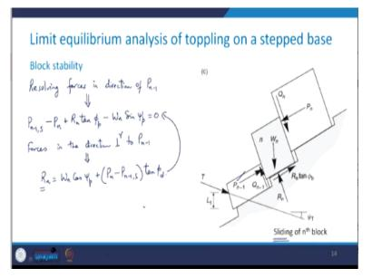
So, how to carry out the analysis? So, what we do is, we resolve the forces in the direction of this ,  $P_{n-1}$ . So, let us do that resolving the forces in the direction of ,  $P_{n-1}$ . What we will get is ,  $P_{n-1,s}$ . Why I am using *s* here because now I am taking the sliding of the n<sup>th</sup> block. So, this is
