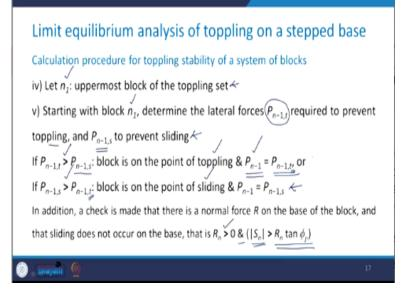
Now, let us say that  $n_1$  be the uppermost block of the toppling set. Now, starting with the block  $n_1$ , we will determine the lateral forces $P_{n-1,t}$ , which is required to prevent toppling and  $P_{n-1,s}$  to prevent the sliding. If the  $P_{n-1}$  value for toppling works out to be more than that for the sliding. This means that the block is on the point of toppling and  $P_{n-1}$  would be assigned the value which is corresponding to  $P_{n-1,t}$ .
