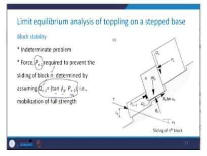
In order to make it determinate, we need to have some kind of an assumption. So, the assumption which is involved here is that force  $P_{n-1}$  which is required to prevent the sliding of n<sup>th</sup> block is determined by assuming  $Q_{n-1} = \tan \phi_d \cdot P_{n-1}$  that means it is assumed that there is the full mobilization of the strength that is going to take place, because if that full mobilization is not there, this condition will not be satisfied.
