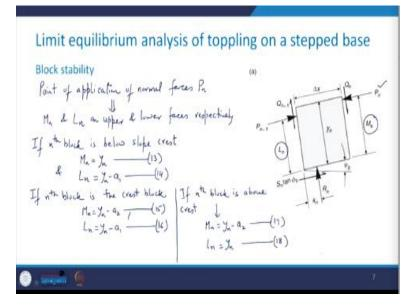
Now, in case of these toppling block, the points of application of the normal forces  $P_n$ , these are given as  $M_n$  and  $L_n$ ; we have seen in the previous figure on the upper and lower faces respectively. See here, this  $P_n$  is acting at a height of  $M_n$  and  $P_{n-1}$  is acting at a height of  $L_n$ . Now, I take the 3 cases that is whether this  $n^{\text{th}}$  block is above the crest, at the crest or below the crest of the slope. So, there is going to be 3 cases.
