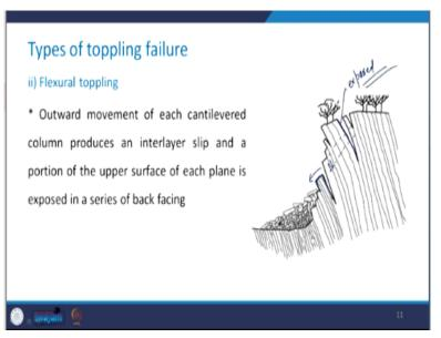
The outward movement of each cantilevered column produces an interlayer slip. So, the moment, there is the outer movement of each column; there is going to be the interlayer slip and the portion of the upper surface of each plane is exposed in a series of back facing. Like you see here, this portion that is the upper portion of this column is exposed in a series of back facing here.
