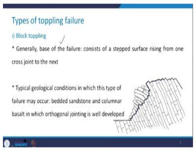
Generally, the base of the failure is consisting of a step surface rising from one cross join to the next. Take a look here, what I mean to say here is that this step portion which is formed by these orthogonal joins of these columns, this is what is going to define the base of the failure surface. Typical geological conditions in which this type of failure may occur involve bedded sandstone and columnar basalt in which orthogonal jointing is well developed.
