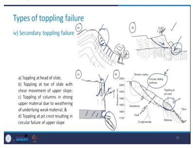
There are few secondary toppling failure which also take place. So, some of these have been mentioned in this figure. So, this portion of the figure which is figure part a, it shows the toppling at the head of the slide. So, you can take a look that here you have the steeply dipping joints and the toppling is taking place at this location. Then here, which is part b, there is the toppling near the toe of slide with the shear movement of the upper slope.
