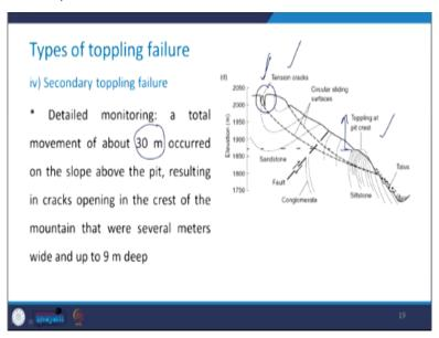
The detailed monitoring of the slope was carried out at the site and the total movement of about 30 meters occurred on the slope above the pit. See here, 30 meter on the slope above the pit that means here above the pit and this resulted in the crack opening at the crest of the mountain which is here; these cracks were several meters wide and up to 9 meters deep these cracks. So, you can see that how one particular phenomena, it triggers the other phenomena.
