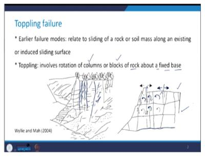
It involves the rotation of the columns or blocks of rock about a fixed base. Take a look at these pictures. And you can see that the rock mass which is here, it has very steeply dipping joints and therefore, it is kind of creating such type of columns in the rock mass and come here and see what it looks like that there is going to be the kind of rotation as shown by these curved arrows of these rock blocks. And this is what is going to happen about a fixed base.
