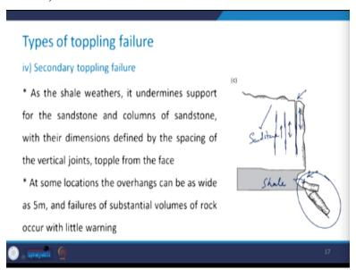
Now, in case of the shale, as it weathers, it undermines the support for the sandstone and the columns of the sandstone with their dimensions defined by the spacing of the vertical joints, they start toppling from the face. So, what this mean is, say, this is the shale and I mentioned to you
