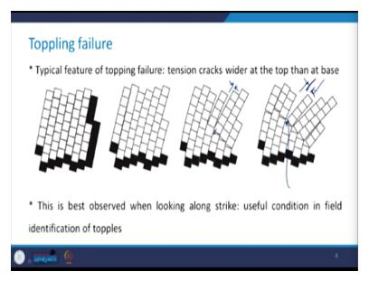
The typical feature of the toppling failure is the occurrence of tension cracks, which are wider at the top than at the base. So, you can see that here the width is only this much. However, here the width is larger as compared to what it was at the base and this is more evident. If you look at this figure, you see here this separation is this much and at the base, it is only this much separation which is there. So, these tension cracks are wider at the top as compared to at the base.
