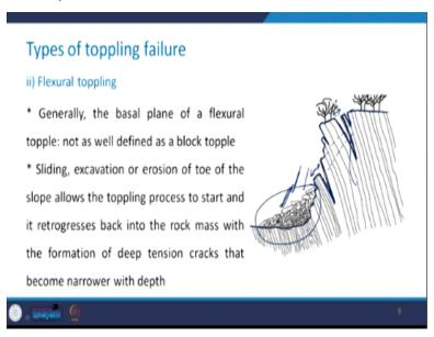
Generally, in this case, the basal plane of a flexural topple is not as well defined as it was there in case of the block topple. You can see here this dark line, this is the basal plane and you can see that it is not very well defined, sometimes there is a separation and then sometimes it is like this. So, it is not very well defined. However, in the earlier case, it was kind of a stepped manner that the base plane verse.
