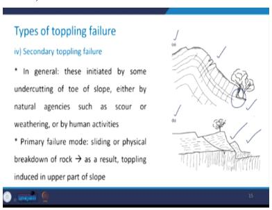
So, I have here a, and b which I explained you earlier. So, in general, these kind of toppling failure are initiated by some undercutting of the toe of the slope either by the natural agencies such as scour or weathering or by some human activities. So, wherever you have the undercutting of the toe of the slope, such type of secondary toppling failure mode can be expected.
