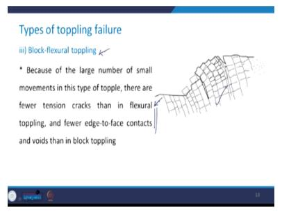
Now, because of the large number of small movements in this type of topple, there are fewer tension cracks than in case of the flexural toppling and fewer edge to face contacts and voids as compared to block toppling. So, the difference between block flexural and block flexural toppling has been given here. In case, if you have this block flexural toppling kind of behavior, there are going to be fewer tension cracks as compared to those which were present in case of the flexural toppling.
