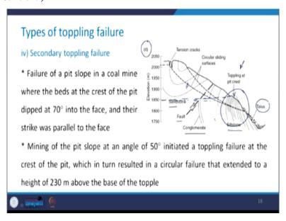
Coming to the last part, which is the type of the secondary toppling failure that is the toppling at pit crest. Now, here you can see that sandstone, fault, conglomerate and siltstones are present as a part of this slope and here you have talus. So, what happens that the failure of a pit slope in a coal mine, where the beds at the crest of the pit, they dipped at 70 degree into the face and the strike was parallel to the face here.
