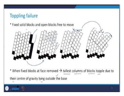
So, these solid lines, they are the fixed blocks and these are all open blocks and these are free to move. Open blocks are free to move. Now, let us say when these fixed blocks at the face, they are removed. So, come from the first figure to the second figure and you will realize that this portion and this portion has been removed in this particular figure. So, you see that what happens is that the tallest columns of the blocks topple due to their center of gravity lying outside the base.
