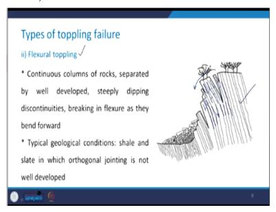
The second type of toppling failure includes flexural toppling. In this case, there are continuous columns of rocks, which are separated by well developed steeply dipping discontinuities. They break in flexure as they bend forward. Take a look at this picture, you have steeply dipping joints
