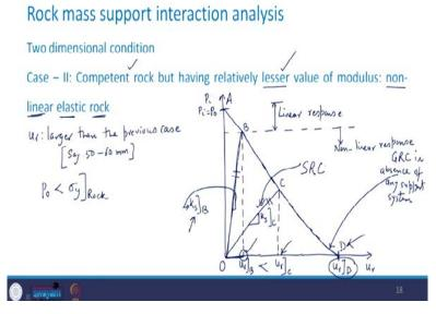
That is it is the non-linear elastic rock. Now, since we know that it is non-linear elastic rock, can we draw the ground response curve? As we did in the previous case, let us try to draw that. So, here on the vertical axis, again we will have the radial support pressure, which is  $P_i$ . And on the x axis, we will have the deformation radial deformation  $u_r$ . Now, in the beginning here, that is the point A as we had in the previous case.
