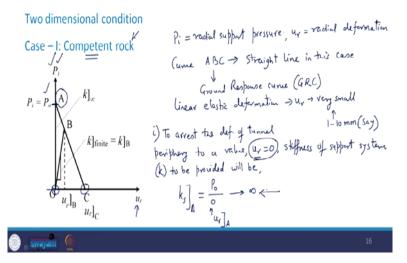
When I say competent rock, what does that mean? That its behavior will be elastic. Now, this  $P_i$  is going to be the radial support pressure. And in this figure you can see that this  $P_i$  has been plotted against the radial deformation, which is  $u_r$ . So,  $u_r$  we are saying that it is the radial deformation. This curve A, B, C in this case of the competent rock, this is the straight line. This is called as the ground response curve. And in short, we call as GRC.
