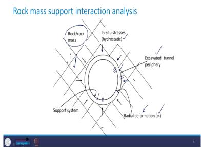
Take a look at this figure. We have rock or rock mass here. Then, this was the excavated tunnel periphery. Then, the support system which has been installed is this one. And there is the margin of this radial deformation which is denoted by  $u_r$ . And here a typical situation of hydrostatic in-situ stress has been shown. That is from the all the direction you have the same stress. So, that is hydrostatic in-situ stresses. So, please understand these terminology.
