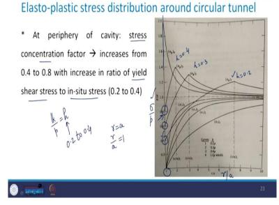
So, at the periphery of the cavity, what does that mean? That is, r=a. So, this ratio r /a equal to 1. And then you can see that here this axis we are plotting r /a. And here it is  $\sigma$ / p. So, this is what is r/a = p. So, we move along this line if you want to see what is the situation at the periphery of the cavity? So, take a look here that this stress concentration factor which has been plotted on this axis, it increases from 0.4 to 0.8.
