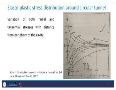
Now, the variation of both radial and the tangential stresses with the distance from the periphery of the cavity has been shown in this figure. Let us try to see some of the typical feature with respect to this stress distribution one by one.
