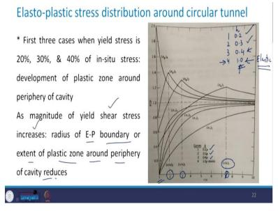
So, here we are taking 4 cases 1, 2, 3 and 4. The first case corresponds to when h is equal to 0.2, second case is for 0.3, third is for 0.4 and the fourth case h will become equal to 1. You can see here that it is written. So, when this is the fourth case as we have seen this is going to be fully elastic situation. So, as the magnitude of the yield shear stress increases, that means for these 3 values you can see as this is increasing from 0.2 times p to p.
