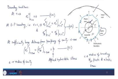
So, we have here boundary conditions. So, take a look at this figure. This boundary that is at r=a. It is the free boundary because here excavation has taken place. So, this is the boundary of the cavity. So, therefore, what we will have here is that
