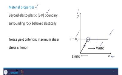
Coming to the material properties, beyond the elasto-plastic boundary, the surrounding rock will behave in an elastic manner. As we have assumed that the rock is following TRESCA yield criterion, which is the maximum shear stress criterion. Take a look at this figure where  $\sigma$  versus  $\varepsilon$  has been plotted up to the elastic limit it goes in a linear fashion in this manner as shown here.
