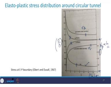
Now, this is the typical variation of  $\sigma_r$  and  $\sigma_{\theta}$  at the elasto-plastic boundary. See this one is for the variation of  $\sigma_r$  at the elasto-plastic boundary. And this is for the  $\sigma_{\theta}$ . While in case of the elastic state, this is the variation for  $\sigma_r$ . And this is the variation for  $\sigma_{\theta}$ . Here on the x-axis you have c/a. And on y axis you have the stress concentration factor as  $\sigma$ /p.
