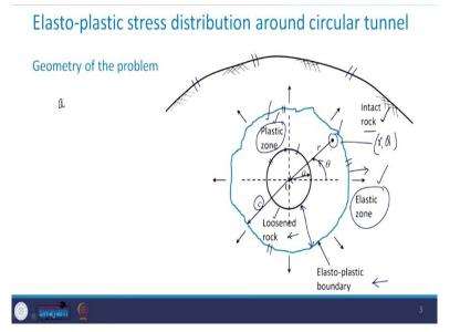
So, this figure shows the geometry of the problem. You see that this is what is the ground condition. Here, this is the intact rock. And in this rock, you have made the excavation in the form of this circular opening which has a radius of *a*. Then, because this rock is in such a way that there is the occurrence of a plastic zone all around this cavity, which is the circular tunnel and that has been represented by this blue colored curve.
