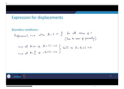
Now, after getting this is the time to apply the boundary conditions. So, we need to apply here the boundary conditions with respect to the displacement. So, what do we have here is that displacement *v* will be equal to 0 then  $\theta = 0$  or  $\Pi/2$  for all values of *r*. Now, what is the reason behind this? It is due to the axis of symmetry. So, this is due to axis of symmetry. Now, this
