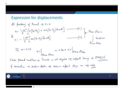
Now what happens at the periphery of the tunnel? That means at r = a. So, at periphery of the tunnel what does that mean? That is r = a,
