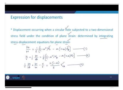
Now what will happen in case of the plane strain, displacement which is occurring when the circular hole is subjected to a two-dimensional stress field under the condition of the plane strain? So, in this case we have to integrate these stress displacement equations which are there for the plane strain. In the previous case we integrated the equations for plane stress. Now from the theory of elasticity what are the equations for the plane strain?
