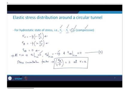
Now, we take some of the special cases and see how the form of the equation 12 becomes for these special cases. So, when we have the hydrostatic state of stress that means, that  $S_x = S_y = -p$  and since it is in compressive in nature, so, I am introducing a negative sign with this state of stress which is *p*. So, what we are going to get if we just substitute this equal to  $S_y$  in equation number 12 what we are going to get is
