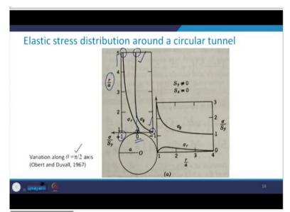
Then focus on this portion of the figure. See here this is at the crown which is at  $\theta$  equal to  $\Pi/2$  axis. So, when you have r/a equal to 1 that means, at r =a that is an eternal periphery, you have  $\sigma_{\theta}/S_y$  to be equal to -1 and we saw that it is like in that condition that a stress concentration factor was coming out to be -1 and that is what has been represented in this figure.
