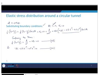
So, in case of this boundary condition in the previous class, we already substituted the boundary conditions, which were at *r* tending to infinity that we did earlier. So, now, we have the other boundary conditions which are like at r = a you have  $\sigma_r = 0$ . Now, when this  $\sigma_r = 0$ , what is the expression that we are going to have is this that is
