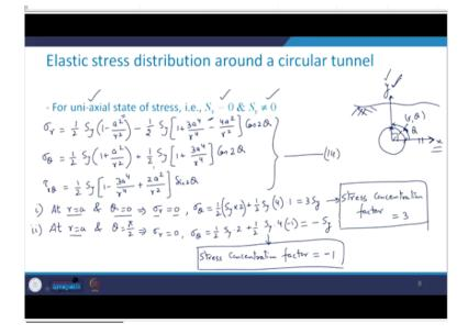
Now, let us take another state of stress which is the uniaxial state of stress in which case I will have a  $S_x = 0$  that means, the applied stresses in the x direction they are 0 and in y direction they have the finite value. So, in such a situation what will happen to  $\sigma_r$ ?
