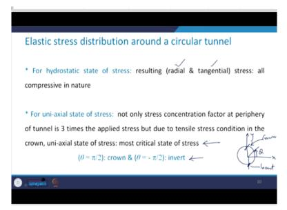
So, we have seen that for hydrostatic state of stress both the radius as well as the tangential stresses. They are all compressive in nature, we saw that the stress concentration factor was all positive in that case. But in case of the uniaxial state of stress, it is not only that the stress concentration factor at the periphery of the tunnel is 3 times the applied stress. But also due to the tensile stress condition in the crown portion of the tunnel.
