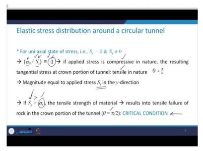
So, here I have summarized what we discussed for the uniaxial state of stress, that is when there is no applied stress in the x direction and only in the y direction these stresses are present. In that case  $(\sigma_{\theta}/S_y)$  we have seen that it is - 1. If the applied stress is compressive in nature, the resulting tangential stress and the crown portion of the tunnel becomes tensile in nature, because you see that the ratio of these 2 is - 1.
