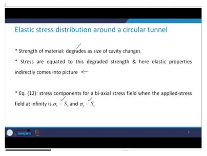
Now, this strength of the material, it reduces as the size of the cavity changes, stresses are equated to this degraded strength and here the elastic properties indirectly come into picture. So, we need to be careful. Equation number 12 which we derived just now, these gave the stress components for a biaxial stress field when the applied a stress field at the infinity is  $\sigma_x = S_x$  and  $\sigma_y = S_y$ .
