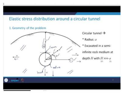
So, to start with look at this figure and here you have this excavation in the form of circular tunnel which has the radius equal to a, that has been shown here, this tunnel has been excavated in a semi-infinite rock medium at a depth H which is this, this is the depth between this point and this point, that is on the ground surface. You need to take a look that this over burden depth is much larger than the radius of this circular tunnel.
