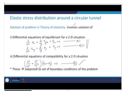
Now, let us try to see how to obtain the solution of this problem using the theory of elasticity? So, basically this involves the solution of first is the differential equation of equilibrium for a 2-D situation, let us see what are these equations? So, we have
