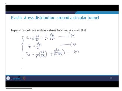
Now, to proceed further in the polar coordinate system, this stress function  $\phi$  is such that
