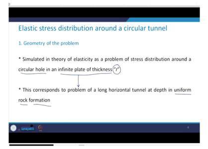
This is simulated in the theory of elasticity as a problem of stress distribution along a circular hole in an infinite plate of thickness *t* and this problem of circular hole in an infinite plate of thickness can correspond to the problem of a long horizontal tunnel at depth in the uniform rock formation.
