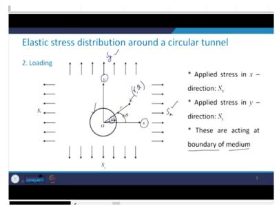
The second aspect is the loading. See this is the tunnel, you have the 2 reference axes x and y. This is the point defined by r,  $\theta$ , where  $\theta$  is the angle in the anticlockwise direction from this x axis, the radius of the tunnel is *a*. Now the applied distress in x direction is  $S_x$  and applied stress in the y direction is  $S_y$ . These stresses they are acting at the boundary of the medium.
