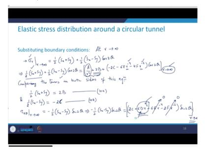
Now, we need to substitute the boundary conditions. So, we have the boundary conditions one was at r tends to infinity and another one was at r tends to 1. So, first let us apply that at r tending to infinity, the boundary conditions are going to be that is
