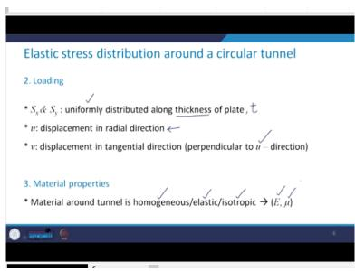
So, this  $S_x$  and  $S_y$  they are uniformly distributed along the thickness of the plate which is *t*, *u* be the displacement in the radial direction and *v* is the displacement in tangential direction which is perpendicular to *u* direction. The third aspect is related to material properties, so it has been assumed that material around the tunnel is homogeneous, elastic and isotropic. So, *E* and  $\mu$  are going to be the material characteristic of rock around the tunnel.
