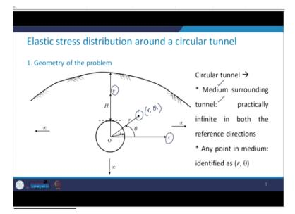
As I mentioned the medium surrounding the tunnel is practically infinite in both the reference directions which are x and y. Any point in the media that is say this point will be defined by the point called r,  $\theta$ .
