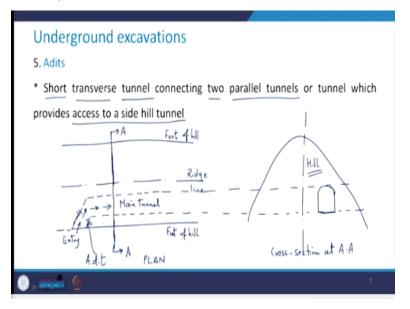
Coming to the next category which are the adits, these are the short transverse tunnel which connect two parallel tunnels or tunnel which provides access to the side hill tunnel. See, this is how it looks like, let us say that in the plan. Say this is a plan where this is foot of hill and obviously this will also be foot of hill. So, I will have here say, a section, say this is a section A, A.
