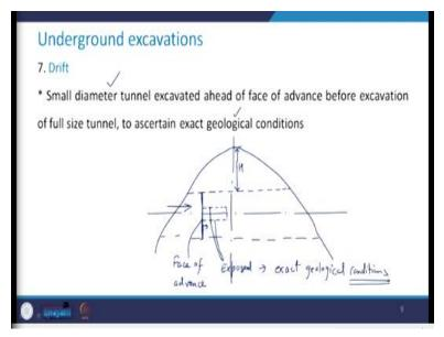
The next one is the drift. Drift is the small diameter tunnel excavated ahead of face of advance before excavation of full size of the tunnel; this is used to a certain exact geological condition. So, in case of the rocks lot of uncertainty maybe there and we may not be aware of the exact geological conditions, from the conditions what are exposed at the surface. So, in order to ascertain about that one needs to go for these small diameter tunnels.
