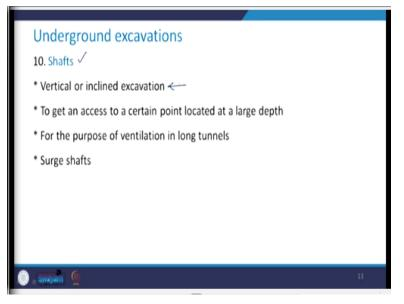
These are vertical or inclined excavation and used to get an access to a certain point located at a large depth. They are also used for the purpose of ventilation in long tunnels; they are used in the case of the surge shafts.
