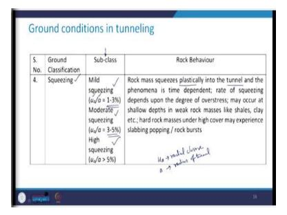
The fourth one and the very important, and these needs a lot of care is squeezing. It has various subclasses, first let us see what do we mean by the squeezing ground condition and then I will explain you that why it is divided into some different sub classes. So, the squeezing rock mass is the plastic, it squeezes plastically into the tunnel and this phenomenon is time dependent. The rate of squeezing it depends upon the degree of overstress.
