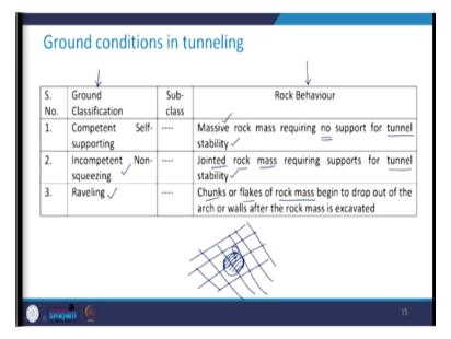
So, here the second column gives you the idea about the ground classification, and the last column talks about the rock behaviour. So, when we say that the ground is competent self supporting, what does that mean? This means that, it is comprising of massive rock mass which requires no support for the tunnel stability. That means if you have the excavation through the competent self-supporting rock, then that tunnel may not need any kind of support for it is stability.
