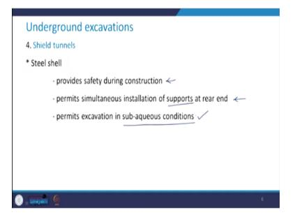
This steel shell will provide safety during the construction; they permit simultaneous installation of supports at the rear end. And also, they permit excavation in sub-aqueous condition that is when in case if you have the tunnel construction in the presence of the water, there are also this help. (Refer Slide Time: 10:08)
