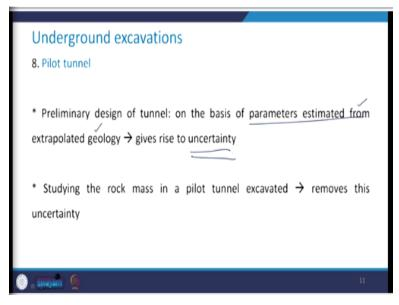
So, as far as the pilot tunnel is concerned the preliminary design of the main tunnel on the basis of the parameters which are estimated from the extrapolated geology, they give rise to the uncertainty. And therefore, studying the rock mass in a pilot tunnel which has been excavated, it removes all these uncertainties. And therefore, this pilot tunnel in the cases where it is really not possible to go for the rock exploration up to that depth is very, very useful.
