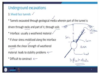
Then you have the third one which is the mixed phase tunnels, till now you have seen that either it was through rocks or you had through the soil or the soft rocks. But in this case tunnels are excavated through the geological media where part of the tunnel is driven through rocks and part of it through soils. So, see it looks like this. Say this is your tunnel cross section and say this is the interface which is continuing on this side as well like this.
