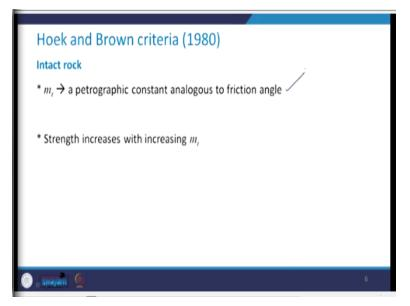
So, basically this  $m_i$  is a petrographic constant which is analogous to the friction angle. And the strength increases with increasing values of  $m_i$ .
