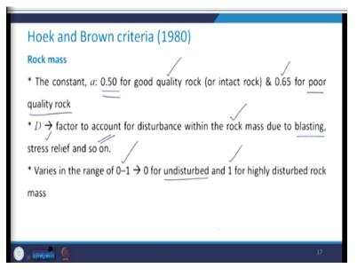
The constant a is 0.5 for the good quality rock or the intact rock, and it takes a value of 0.65 for poor quality of rock. As mentioned, D is a factor to account for the disturbance within the rock mass due to blasting stress relief and other such phenomena. And it varies in the range of 0 to 1, 0 for the undisturbed rock mass and 1 for the highly disturbed rock mass.
