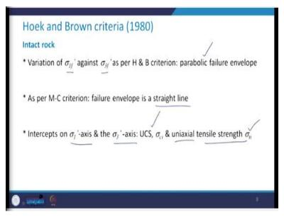
So, as I mentioned it is variation of  $\sigma_{1f}$  again  $\sigma_{3f}$  as per Hoek and Brown criterion is the parabolic failure envelope. In case of the Mohr coulomb criterion, it was a straight line and the intercept on  $\sigma_1$  axis and the  $\sigma_3$  axis gave us respectively UCS of the intact rock and uniaxial tensile strength of the intact rock.
