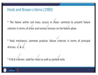
The failure within the soil mass, it occurs in shear, we all know this. And therefore, it is common to present the failure criterion in terms of shear and the normal stresses on the failure plane. But in case of rock mechanics, it is the common practice to represent the failure criterion in terms of principal stresses which are  $\sigma_1$  and  $\sigma_3$ . It is the convention to represent the major principal stress by  $\sigma_1$ , and minor principal stress by  $\sigma_3$ .
