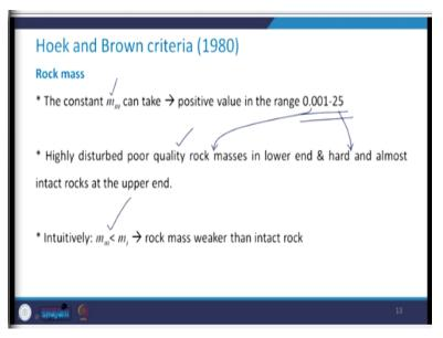
Now this constant  $m_m$  which is for the rock mass, it can take the positive value in the range of 0.001 to 25. Highly disturbed poor quality rock masses they will fall towards the lower range and hard and almost intact rock will be at the upper end. Intuitively we can say that because of the fact that rock mass they are weaker than the intact rock. Because of the presence of the discontinuity, intuitively  $m_m$  will be less than  $m_i$ .
