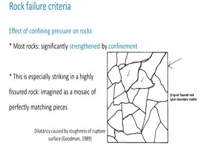
So, a highly fissured rock can be imagined as a mosaic of perfectly matching pieces like it has been shown in this figure. You can see that these are the planes of the discontivity in case of your fissured rock and these discontivity planes they are matching perfectly with the next piece. So, let us say this is one piece, this is another piece, so it is matching with this other piece in a very nice manner.
