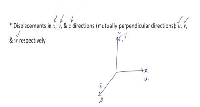
So, the strain in the elastic body they are caused by the displacement. So, there should be a relationship between strain and displacement and we should be aware of that. So, let us say that displacements in x, y and z directions they are respectively u, v and w. So these x, y, z these three directions they are mutually perpendicular to each other. So, let us say this is your x, this is y and this is going to be z.
