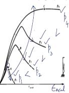
Now another aspect that what happens when we increase the confining pressure or we are calling here as mean pressure. Have a look here, there is a plot between  $\in$  axial and  $\sigma 1 - p$ , p is being represented as the mean pressure which is nothing but the confining pressure. And you can see that the 4 plots are there, they are corresponding to the mean pressure of p 1, p 2, p 3 and p 4.
