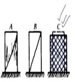
So, at the pressures above brittle-to-ductile transition, there is not going to be any failure because the material is behaving in a ductile fashion. But the deformed specimen is found to contain parallel inclined lime which are the loci of intersection of the inclined rupture surfaces and the surfaces of the specimen that is the condition vmber C. So, you can see here that you are getting these two sets of inclined lines which are intersecting the surface of these specimens.
