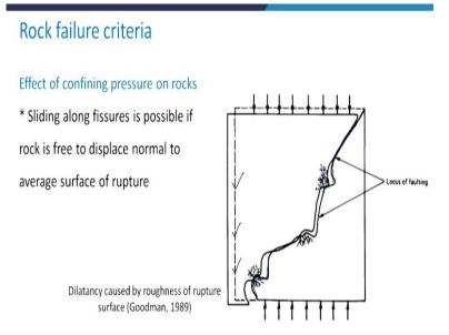
Say for example you can have any fracture plane along any of the combination which is shown here in this figure. So, you see that a typical fracture plane has been shown here. So this dotted line portion that is this portion is the original version and now you see when the load is applied, so sliding along the fissure is possible only if the rock is free to displace normal to the average surface of rupture.
