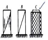
Now the examination of the deformed rock will show intracrystalline twin gliding, intercrystal slip and finally the rupture in such situation. Now Mogi in 1965 he talked about this brittle-to-ductile transition pressure and suggested that when your  $\sigma 1 - \sigma 3$  is approximately equal to 3.4 times the confining pressure or  $\sigma 3$ . Then this condition, this stress state will correspond to the brittle 2 ductile transition.
