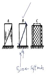
Now when you increase the confining pressure, the failed specimen it demonstrates faulting with an inclined surface of rupture which is traversing the entire specimen. Take a look at the
