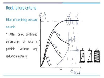
After the peak the contived deformation here in this case, see here after the peak in all these three cases there is a sudden reduction and this is less striking when you are increasing the value of p. But when the ductile behavior is there that is in this case, so the contived deformation is going to take place, so you see that this is after c. That means c is the point kind of a peak and beyond this the contived deformation of the rock is possible without any reduction in the stress.
