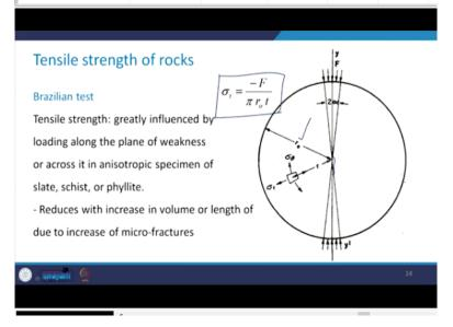
As a schematic diagram, as I mentioned that the specimen should be loaded along the diameter and this is valid when the crack starts propagating from the centre only along this diameter. So, this is the philosophy. So, this tensile strength can be determined by this expression,
