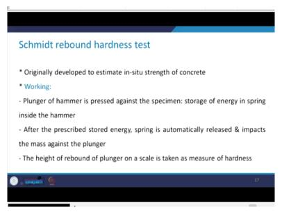
Now, coming to the next test, which is useful in order to obtain the compressive strength of the rock and it is very simple. That is called as Schmitt rebound hardness test. This was originally developed to estimate the in-situ strength of concrete. What exactly is its working? So, there is
