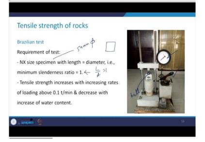
So, the test requirement for the specimen it should be the NX size specimen. Now, what is the typical characteristic of NX size specimen? That it has 54 mm diameter, now with L/d ratio to be equal to 1. So, minimum slenderness ratio L/d we will take us 1 in this case again. So, it will be something like this, this tensile strength increases with increasing rates of loading above 0.1 tonne per minute.
