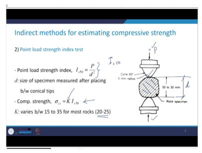
As I mentioned, this is the line sketch. Here is the rock specimen, this one which may have the dimension from 30 mm to 50 mm and you have the loading platen as the cones which are having  $60^{\circ}$  apex angle and then here it is, this is 5 mm radius. You apply this point load here, which is capital P. So, the point load index is defined as
