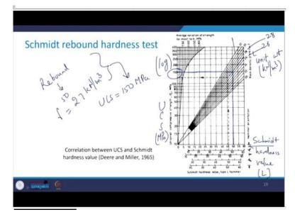
See here that you have the correlation between UCS and Schmitt hardness value. So, this is given for the L type hammer. So, on this axis here you have UCS in MPa. And these radial lines, these are giving the unit weight of the rock in  $kN/m^3$  and this axis gives us the Schmidt hardness value and this is for L type hammer. Now, how to read this?
