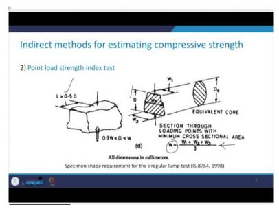
Similarly, if you have the irregular lump test, so, in that case again this length requirement remains the same and its cross section if you see, it is not constant along this dimension D. So, what you need to do is you take the average dimension in this direction, so, that you can obtain as W 1 + W 2 + W 3. That means, you measure it at the top at the bottom and at the middle,
