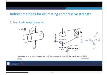
Now, in case if we have any other shape of the specimen, then the code that is IS:8764 gives us some of the shape requirement for the specimen for different shapes of the specimen. So, let us say that, for the diametral test, when I say diametral test means the loading is applied along this diameter and the length of the specimen or the loading point should be more than 0.5 times its diameter from one end as has been shown here.
