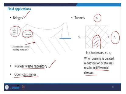
Then the next one bridges; you can see here there is a foundation and anchor block. And then discontinuities are there which have been shown by this arrow and until unless we know the orientation what is the type of the rock etc., I cannot go ahead with a proper design of these foundation or anchor block or abutment for bridges. So, in case of bridges, it is equally important for us to know about this subject that is rock engineering. Then come to tunnels.
