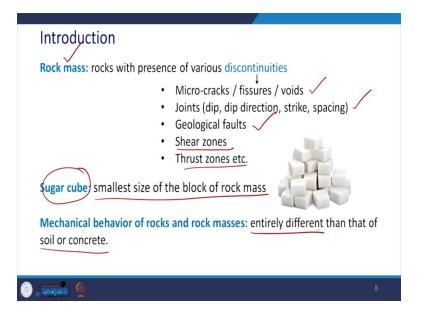
Now these discontinuities can be in the form of micro cracks fissures or voids they can be in terms of joints it can be geological faults, it can be shear zones or thrust zones then we call that as rock mass. Please remember that rock with the presence of various discontinuities is called as rock mass. Now you know this you come across this rock mass every other day in the form of sugar cube. So, you see that here I have just put a picture where these sugar cubes are there.
