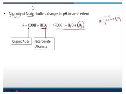
As I mentioned, alkalinity of the sludge is very much important, why is that? Acetic acid, so as you can see organic acids or even acetic acid that are going to lead to soaring of anaerobic digestors. There is a term called soaring, so that is one aspect to keep in mind. Here you have HCO3- the one that is going to be prevalent at pH 7 or near around pH 7, the inorganic carbon that can be take up H+.
