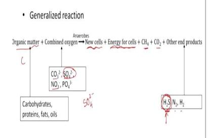
Lets just look at the generalized reaction, so you have the organic matter carbohydrates, proteins substrate and source of carbon. And what is typical electron acceptor? It can be suphates, nitrates, carbonates or such. And anaerobes, what are they going to use it for formation of new cells? Energy for these cells they have to thrive for one is reproduction, one is the energy for this cells being functioned.
