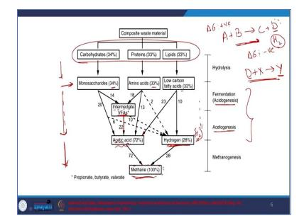
First I have relatively more complex organics here. And this is by COD, this percentage is by the total COD so initially I have 100%. After hydrolysis, I am going to have relatively simpler organic compounds, you can see the COD is still there. And then what is it that being formed? In the acedogenesis, you are going to have intermediate volatile fatty acids being formed.
