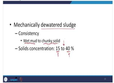
Mechanically dewatered sludge the one that we just looked at we know the consistency it is like wet mud or chunky solid, what we looked at the output from the belt press that we looked at is somewhere in between and for wet mud 15%, chunky solids 40%. Ours would have been somewhere in between, there are different ways to look at it. We will look at all these aspects.
