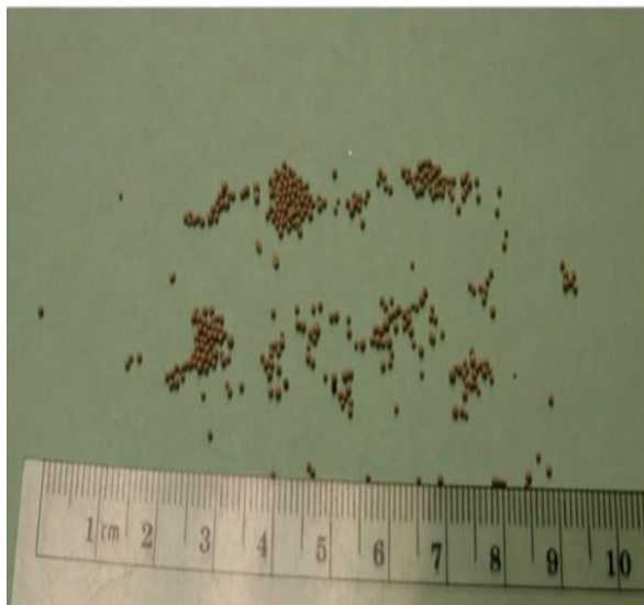
Ion exchange resin beads (500-590 \mu\text{m} diameter)
