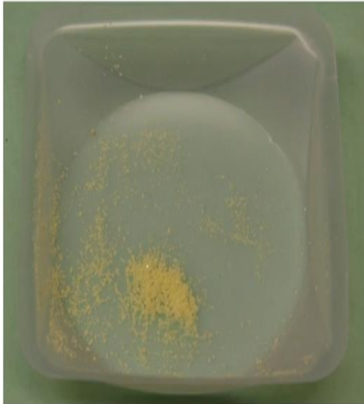
Ion exchange resin beads (75 -150 \mu\text{m} diameter)
