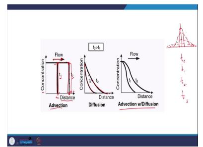
Just to understand, if we have just advection how is it going to look like and if it is advection diffusion, and so forth, how is going to look like. Here we have concentration and distance, and if I put in a tracer at one particular point or such, and at time  $t_1$ , the concentration is out here. At time  $t_2$  also the same plug will move and the concentration at time  $t_2$ , or the distance  $X_2$  here we are talking about distance.
