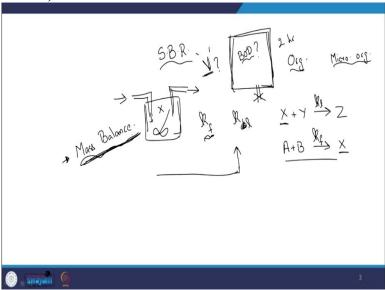
As we looked at earlier, we saw the video of a wastewater treatment plant in that video we had what we looked at was a sequential batch reactor. Let us say are about we look at the details later. We have this particular reactor fine, and we had water coming in, and then it is filled to a particular threshold and then we turn off the inlet flow and then aeration occurs where during which microbes degrade your substrate or the organic compounds.
