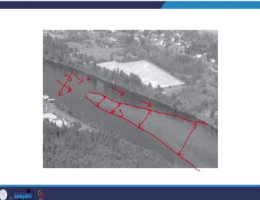
In the next example that we are going to look at, I am not sure if it is remarkably clear, but as you can see, through an underground diffuser, or the diffuser at the bottom of the canal, you see that the waste is being given out here. But unlike the previous slide that we looked at, we see that with time, this width of this waste is increasing? Here, it is X here, it is maybe 2X, and so forth.
