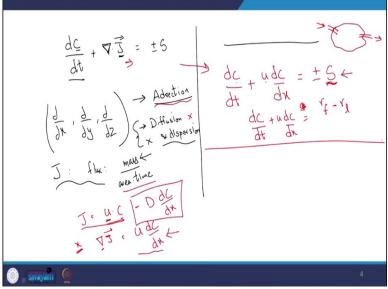
For that, what do we need to do? Before I go further to that slide, note that in this class, we are going to use one approach for fundamental or for mass balance, and we look at that equation. But before I do that, I would like to acquaint you with the fundamental mass balance equation. dc / dt, c is the concentration of the compound, the interest, plus the del product of the flux is going to be equal to plus or minus sources and sinks.
