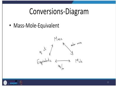
Let us move on what else do we have? Conversion, I will just talk about this diagram and we will move on I have mass I have moles and I have equivalents. How can I interconvert mass to moles, I need to have the molar mass either divide or multiply and here I will have to have the equivalent weight or the equivalent mass. Here I will have to have equivalents per mole, which so in that way, I can convert from one unit to the other. I just wanted to mention that.
