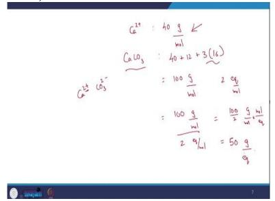
For example, Calcium, molecular weight, how much is that? 40 grams/mole, and with respect to  $CaCO_3$  40 + 12 + 3 into 16. This is 48 and 16. That is going to be equal to 100 grams per mole. Here, we are looking at it with respect to charge and pause to charge at  $Ca^{2+}$  and  $CO_3^{2-}$ , so +2 charge out here so based on that, you can calculate the equivalent weight.
