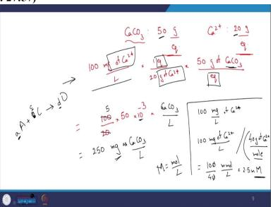
Let us just write that out. I have a CaCO<sub>3</sub> the equivalent weight was supposed to be 50 gram per equivalent, and here we are talking about charge, keep that in mind equivalent in terms of charge, and for Ca<sup>2+</sup>, we said that it was going to be 20 gram per equivalent and the concentration I have is 50 milligrams of Ca<sup>2+</sup> per liter of this water. Here, I want to convert this into equivalents.
