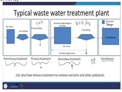
Preliminary treatment, where plastics, tree leaves, branches are removed out here bar screens and grit chamber will have good pictures later. Primary settling relatively bigger particles, quite a few wastewater treatment plants sometimes do away with this primary treatment, and then you have the biological process again here we have the sludge but for the sake of easier understanding I removed it out here.
