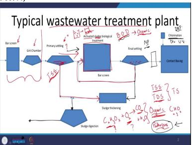
Wastewater treatment, I have water that is high in total suspended solids, has some dissolved solids, total dissolved solids, the some of which will be total solids, and typically the issue is that it will have a lot of organic content, CHO, xyz stoichiometry, and this when I release into the oceans, what is going to happen to this organic content? The surface water bodies are such, it will undergo degradation.
