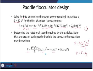
We are done with some aspects. Then we will check the design the different way. Solve for P now. I need to know the power from the G that is given . What it is?  $P = G^2 \mu V$ . I have G; I
