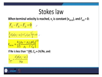
So, we can balance them out, put in the relevant terms and get the relevant, , equation and for terminal velocity, this is the equation, . , this is first spheres and we are assuming that the conditions are laminar flow. So, that is why we are saying that Reynolds number less than 1. And as you can see, coefficient of drag will also depend upon the relevant flow conditions. Yes. So, that is what we see, let us move on.
