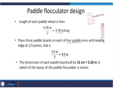
So, the length of each paddle will be 6.36 by 2. So, until now, what do we have? We have the width; we have the length; we know the clearances; we know that it is going to be 2 and each one is going to be, the diameter is going to be 3.18 metres, . At the length of each paddle wheel, there is depending on how you are going to mention it. So, place 3 paddle boards on each of 4 paddle arms.
