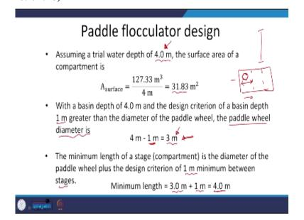
Let us move on. So, trial water depth, 4 metres, the surface area then will come out to be volume by depth that is going to be 31 metre square. Trial, typically decent value not too high and certainly not too low considering the paddle vet. Yes, with the basin of 4.0 metres and design criteria, which was presented in the table previously, of basin depth one metre greater than the diameter of the paddle wheel.
