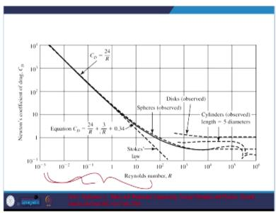
And it also depends upon the type of flow conditions. Yes. So, typically, Reynolds number one or less, what do we call that, we call that laminar flow conditions. And for laminar flow conditions, first spheres, stokes law is applicable.
