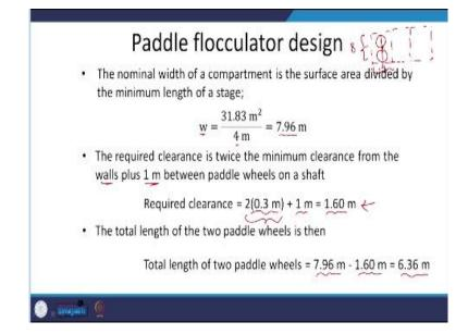
So, if we have the length, I can calculate the width from the area that we had earlier. Area by length, this is the width. So, what did I calculate? I just calculated the, so, this is my compartment, yes, so, this came to be 4 and this came to be almost 8 metres or 7.96 metres that is what we calculated and the required clearance is twice the minimum clearance from the walls plus 1 metre between paddle wheels on a shaft. There is some more to go.
