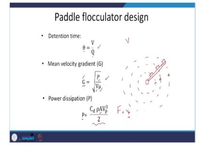
Let us look at the 3 formulas that we typically use. , dimension time, we covered this. Mean velocity gradient, yes, we already covered this. So, depending on the question, you will go from either the power to calculating G or from G to calculating power, . So, here, what is it that I am doing? First, I will, what is the approach? What is the overall approach? First, from the given theta and Q, I will calculate the volume.
