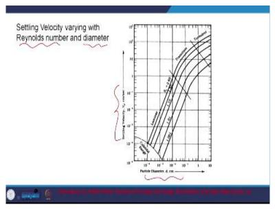
And settling velocity will vary with both the Reynolds number and the diameter . So, here we see that for our particles of interest, which are relatively lesser, they will settle under laminar flow conditions. And you can see that , because the size is lesser, their settling velocity is also relatively small. And , with specific gravity, this is specific gravity. So, heavier particles will settle faster that is something that you can see out here.
