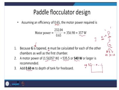
So, let us move on. Assuming an efficiency of 0.65. This is what we assumed as not all the power from the motor is going to be transferred to the water while the paddles. So, here we are assuming that the efficiency is 0.5. So, motor power required is the relevant aspect.
