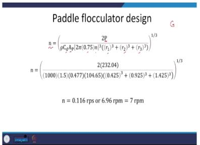
So, this is the radius we are looking at and from that, I will get the n or the rotational speed that I have to maintain. Power, we calculated that from the G that we required, yes, area of the paddle from the length and width, coefficient of drag given and then k 0.7 and rotational speed, we have to calculate r 1, r 2, r 3; we calculated. So, from that you solve for n. So, it comes out to be these many revolutions per second or 7 revolutions per minute.
