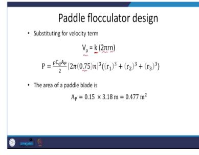
So, velocity of the particle, this particular constant  $2 \pi$  r; the perimeter it is going to cover and rotational speed. So, the constant we are taking, is 0.75. This will give me an idea about the velocity of I mean, the paddle relevant to the water by relevant to the fixed coordinate. So, that is something to keep in mind. In general, we are taking it 0.75 and then we are taking it out to be common.
