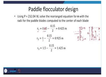
And using power, we already have the power and radius, we can calculate r 1, r 2 and r 3. So, this is based on the fact that we have at that 0.5 metre spacing, . So, 0.15 minus of this should have been 0.5 pardon me, -0.15/2 if I am not wrong, yes. And 1-0.15/2, 1 minus 0.15. Why 0.15? Because, this width of each is 0.15 and this one is point, , this leading edge was supposed to be 0.5, this was 0.5, this leading edge or , this should have been the leading edge, let me redraw that.
