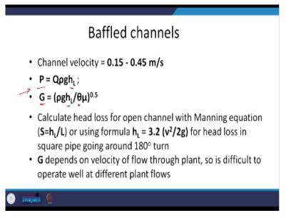
So, you have channelled velocity, power and depending on head loss, you can equate them. This is something we already looked at for the static mixers, when we looked at the power dissipation. So, from that you can equate the level of mixing to the head loss and the retention time. So, that is something that you can get. So, how do we get this head loss or such?
