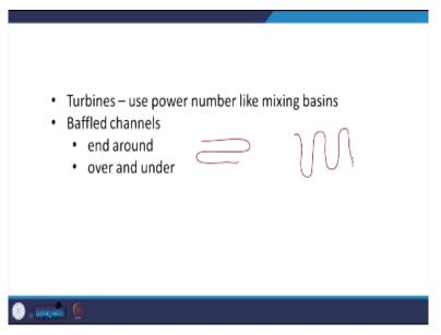
So, let us look at the other aspects to turbines, they use power number like the mixing basins, baffle channels, we already looked at looked at it and around or over and under; over and under This will create the gentle mixing conditions. Baffled channels.
