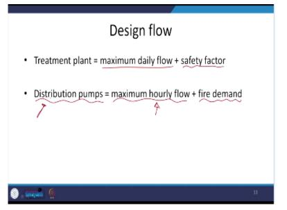
And design flow at the treatment plan, what treatment plan, what is it that we look for maximum daily flow and some safety factor, but with respect to the pumps, what do they need to be able to calculate or look at maximum hourly flow. This is with respect to hourly flow and more importantly to need the fire demands. So, this is something that we need to consider especially when we are looking at the distribution pumps or OHT, . Let we move on. (**Refer Slide Time: 33:42**)
