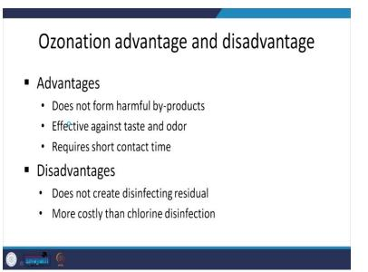
So advantageous in general does not form harmful DBP's very effective st taste and water causing compounds and because of its fast kinetics and relatively high oxidation potential you are going to have less contact time. But does not create disinfecting residual why because it is so fast acting the kinetics are so fast of this particular accident that it does not stay in water for long.
