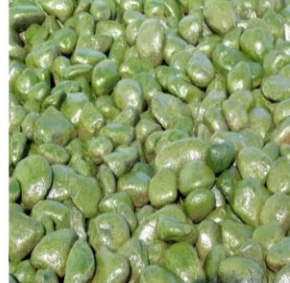
b) Filter media with biofilm
