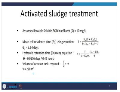
So let us look at the relevant approach. So at the end of the day I need to be able to calculate volume. Volume is  $\theta$  times Q. So in that question I should have also asked to calculate  $\theta$ C. So in this question I want to calculate  $\theta$ C and volume. Volume for that I need  $\theta$  - hydraulic retention time this gives me an idea about how much time the water molecule is spending in the system.
