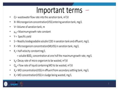
So terms we looked at this and we would also have added some more terms. So Q will give me an idea about how much or the rate at which the water is flowing into the tank volume per time. So volume per time Q flow rate. X as mentioned here it will give me an idea about the microorganism concentration in the relevant tank. So MLSS, MLVSS that is how we typically measure that.
