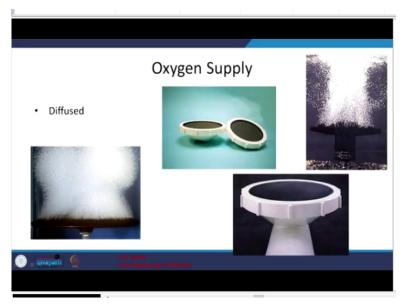
different types of diffusers are available. diffused so you want to create these kinds of fine bubbles or sometimes coarse bubbles which I am not going into detail now.
